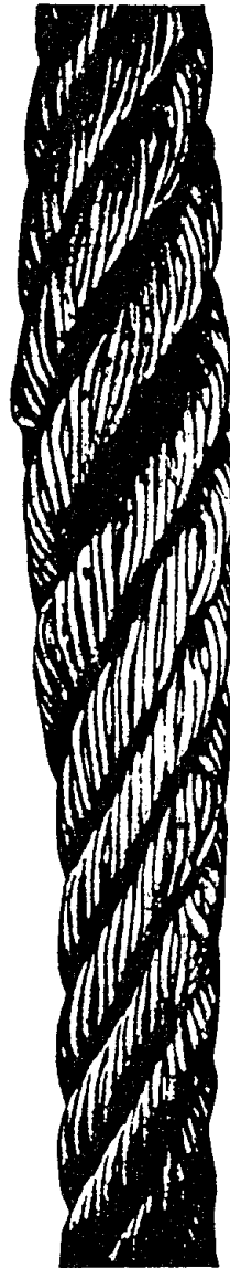
Localized crushing of rope
