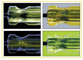
FIGURE 3: What you can see depends on the light you shed on the object. Different types of illumination can solve or create problems for your imaging system.
