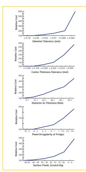
FIGURE 4: The effect of relative costs are shown for various parameter and tolerance specifications. The value 100 represents the cost of a basic element.
