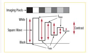
FIGURE 3: Contrast is the difference in intensity between blacks and whites. For an image to appear welldefined, black details must appear black and white details must appear white. The greater the difference in intensity between a black and white line, the better the contrast. The human eye can see a contrast of as little as 1-2%. A typical limiting contrast of 10 to 20% is often used to define the resolution of a CCD imaging system.
