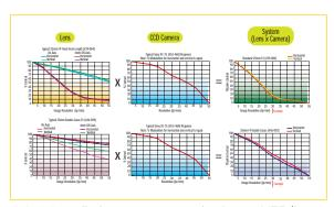
FIGURE 6: Each system component has its own MTF (lens, camera, cables, capture board, and monitor). Multiplying each MTF yields an overall system MTF.
