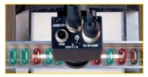
FIGURE 1: An application where multi-colored pills are sent down a conveyor belt and sorted via an imaging system.
