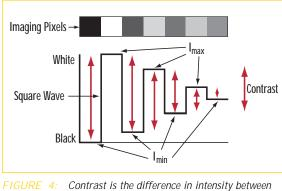
blacks and whites. For an image to appear welldefined, black details must appear black and white details must appear white. The greater the difference in intensity between a black and white line, the better the contrast. The human eye can see a contrast of as little as 1-2%. A typical limiting contrast of 10 to 20% is often used to define the resolution of a CCD imaging system.
