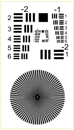
GURE 2: Two test targets: a bar target and a star target allow users to measure resolution and astigmatic errors.
