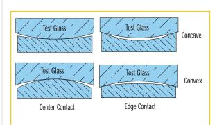
FIGURE 5: Polishing on the "low side".
