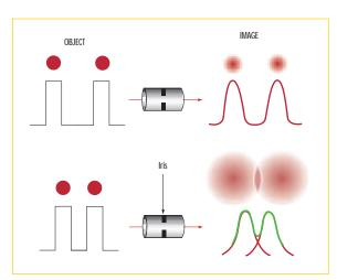
FIGURE 5: Contrast is not constant; it depends on frequency. The dots at the top of the figure can be imaged through a lens. They blur slightly. If we moved the spots closer, their blurs overlap and contrast decreases. When the spots are close enough that the contrast becomes limiting, that spacing is our resolution.
