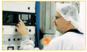
FIGURE 3: A technician sets specifications on a coating chamber. A labor- and time-intensive process, coating deposition involves nine separate steps.
