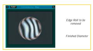
FIGURE 3: Interferogram of PCX lens showing "edge-roll".
