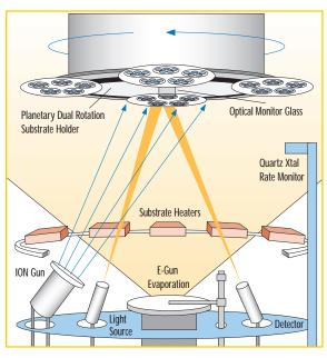
FIGURE 2: Coating chamber subsystems, from top to bottom, may include planetary tooling that holds the components, a quartz crystal deposition rate monitor, substrate heaters, ion-beam gun, e-beam system for vaporizing material from targets and depositing the material onto the components, and an optical deposition rate detector (including the light source and detector).
