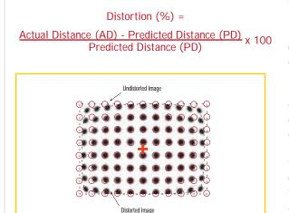
FIGURE 3: Calculating the Actual Distance (AD) and Predicted Distance (PD) for barrel distortion.
