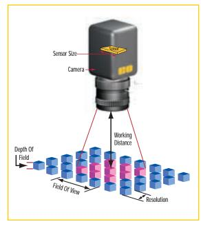
IGURE 1: The fundamental parameters of an imaging system include the resolution of the object, the field of view, and the depth of field the user wishes to image. The sensor size and the working distance from the object to the lens are also important. The primary magnification is the field of view divided by the sensor size.
