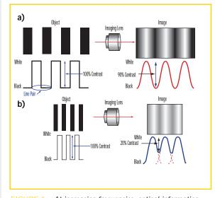
FIGURE 1: At increasing frequencies, optical information passing through a lens loses contrast. (a) The 100% contrast information becomes 90% contrast. (b) The higher-frequency information that starts at 100% contrast becomes 20% contrast after passing through the same lens.
