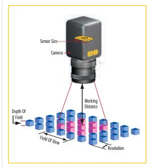
IGURE 1: Fundamental parameters of an imaging system include the resolution of the object, the field of view, and the depth of field that the user wishes to image. The working distance, from the object to the lens, is also important, as is the sensor size. The primary magnification is the field of view divided by the sensor size.
