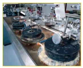
FIGURE 2: Many elements are blocked onto one tool and ground and polished at the same time.
