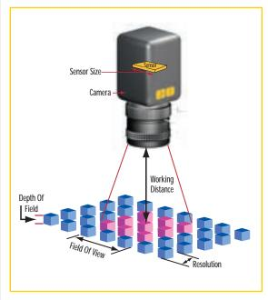
FIGURE 1: Fundamental parameters of an imaging system.
