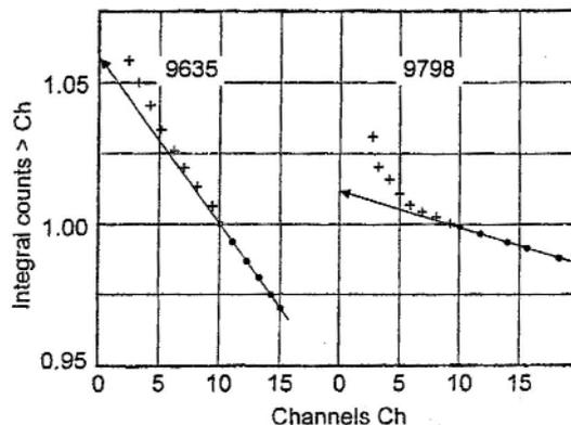
**figure 3** integral pulse height distributions showing contributions from low channel numbers, +, a determined from measurements made at higher tube gain. The ordinate is normalized to the number of counts  $\geq 10$ .
