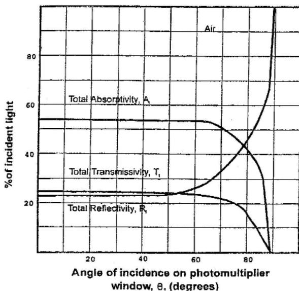
**figure 4** measured optical parameters at 442 nm for an Electron Tubes 9124B illustrating why the quantum efficiency depends on angle of incidence [17]. This paper also has curves for photomultipliers immersed in water.
