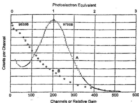
**figure 2** single electron pulse height distributions for: (A) a linear focused multiplier with a well resolved peak; (B) a venetian blind multiplier without a peak.
