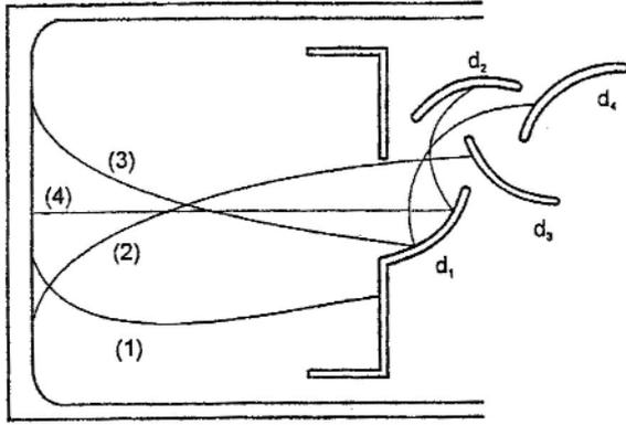
**figure 1** electron optics of a photomultiplier front-end showing how photoelectrons get lost.
