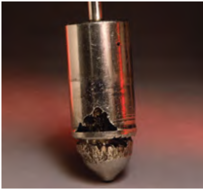
Figure 5.8 Typical Appearance of Flashing Damage
