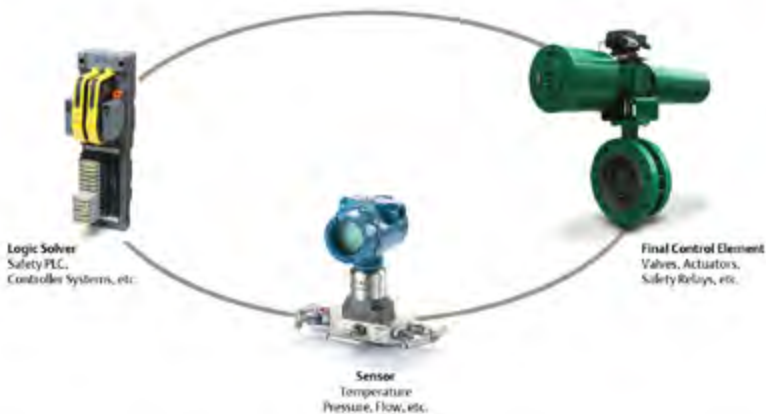
Figure 12.2 Components of a Safety Instrumented System (SIS)
