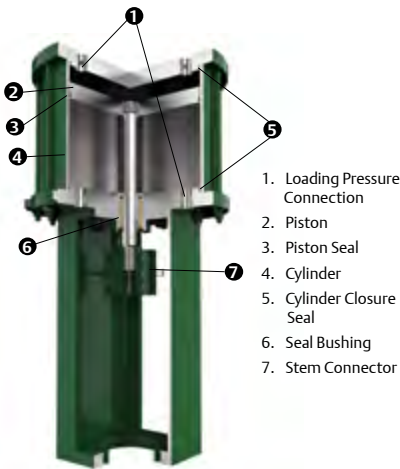
Figure 1.10 Piston-Type Actuator
