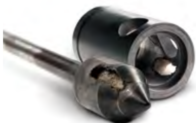
Figure 5.9 Typical Appearance of Cavitation Damage
