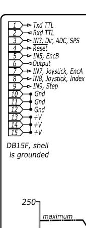
Note! all signals are TTL(+5v). Maximum allowable voltage is +5.5, minimum is -0.5. Do not connect RS232  $(\pm 10v)$  signals directly. For interface to RS232 PCs, use our RS232-TTL Adaptor, which translates the  $\pm 10v$  to +5v logic.
