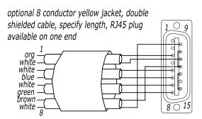
Simple Serial Bus provides a daisy chain "network" to connect multiple Controllers. The PC is the Master and each FTFc15 must be set to a slave address. You must first set the address for each Controller **before** connecting this daisy chain. The transmit pin of each Controller is tied to the Receive pin of the next Controller. See the Excitron Controller
