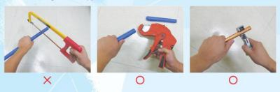
Do not use a hacksaw to cut a pipe. Do not leave burrs on the pipe.
