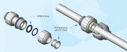
Ensure that the tubing is pushed into the fitting fully past both the collets (gripper) and the '0' ring and is engaged properly in accordance with the manufacturer's instructions.
