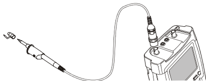
Figure 51. HF Voltage Probe Connection Using Ground Spring
