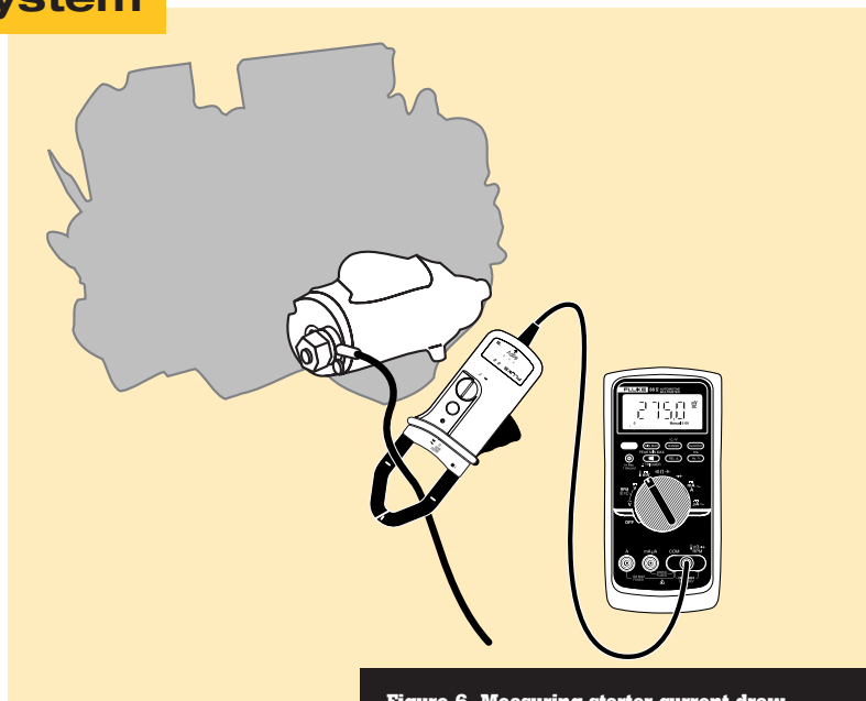
Figure 6. Measuring starter current draw
