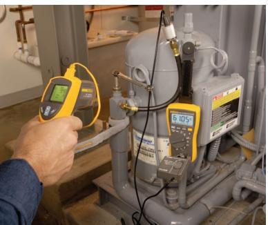
Measuring temperature and suction pressure to determine superheat.
