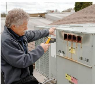
Testing roof-top refrigeration system with a Fluke 561 Infrared Thermometer.
