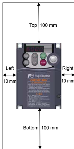
Figure 2.1 Mounting Direction and Required Clearances
