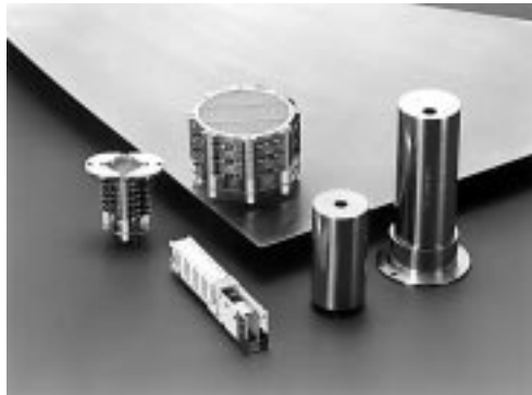
Figure 5-1: Electron multiplier tube structure
