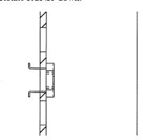
Cage nut fully positioned
