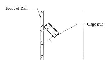
STEP 1: Locate cage nut as shown on back side of rail.
