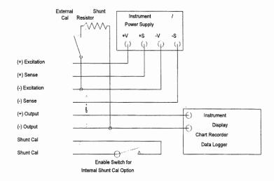
I.EXCITATION: The voltage being supplied to the transducer across the excitation terminals.
