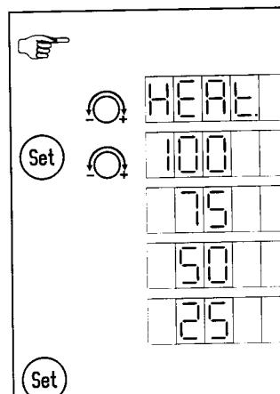
In case of need call up the function menu (see 2.1). Turn the rotary knob until the message *Heat* appears. Confirm with set key.
