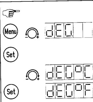
In case of need call up the function menu (see 2.1). Turn the rotary knob until *Deg.* is displayed. Select the function with the Set key.
