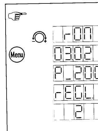
In case of need call up the function menu (see 2.1). Turn the rotary knob until *Rom* is displayed. Confirm with set key.
