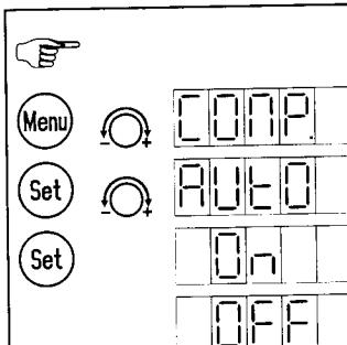
In case of need call up the function menu (see 2.1). Turn the rotary knob until *Comp.* is displayed. Confirm with set key.
