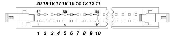
Figure 7-16. Scanner Pin Scan Order For A 20 Pin DIP Package.
