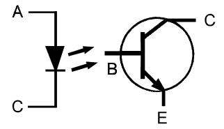
Figure 5-41. Diagram Of An Optocoupler.
