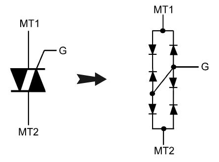
Figure 5-51. Diagram And Symbol Of A TRIAC.
