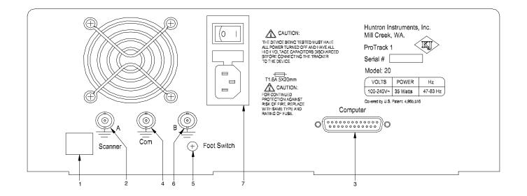
Figure 2-3. ProTrack Model 20 Back Panel.
