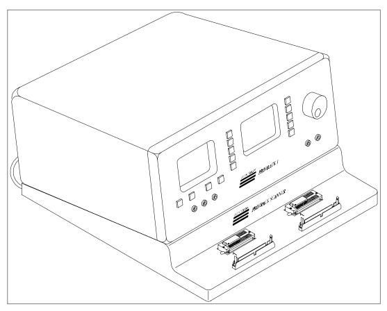
Figure 7-5. ProTrack Scanner With DIP Components In ZIF Sockets.
