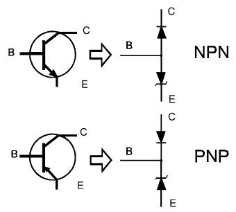
Figure 5-21. NPN And PNP Bipolar Transistors' Equivalent Circuits.
