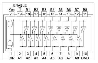
Figure 6-1. Digital IC 74LS245 Block Diagram.
