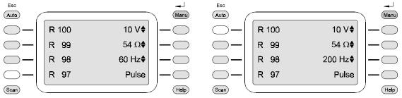
Figure 3-19. User Range With Frequency = 200 Hz (Selected).
