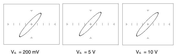
Figure 4-29. Affect Of Varying V<sub>s</sub> On Inductor Signatures. LOW Range,  $F_s = 60$  Hz, L = 12,000  $\mu$ H
