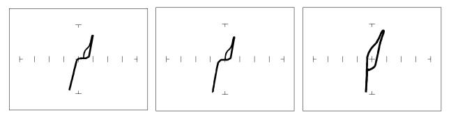
Pin 1 Input - MOS1 range Pin 2 Output - MOS1 range Pin 14 V<sub>CC</sub> - MOS1 range Figure 6-9. Signatures Of A 74HC14 CMOS Hex Inverter. MOS Group
