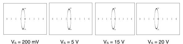
Figure 4-19. Signatures Of A 1 µF Capacitor At Different Test Signal Voltages. MED2 Range (Factory group)
