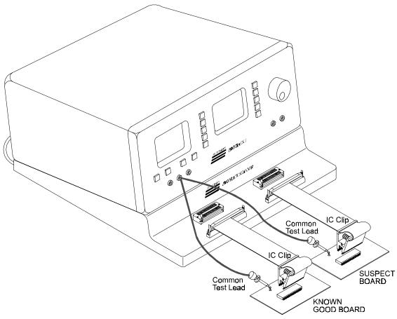
Figure 1-2. ProTrack With Protrack Scanner.
