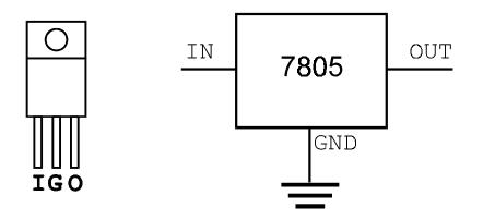
Figure 6-17. Diagram And Symbol Of A Linear Voltage Regulator, 7805 Type.
