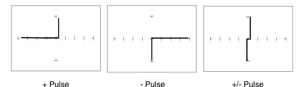
Figure 5-53. TRIAC Signatures With The Pulse Generator Test. MED2 (Factory Group), PW (Pulse Width) = 50%.
