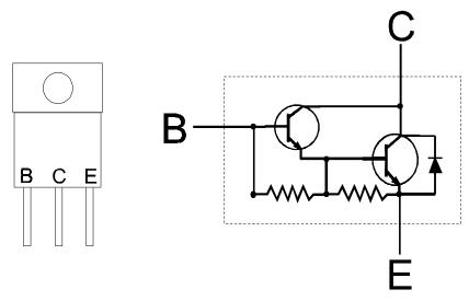
Figure 5-31. Diagram Of A Darlington Transistor.
