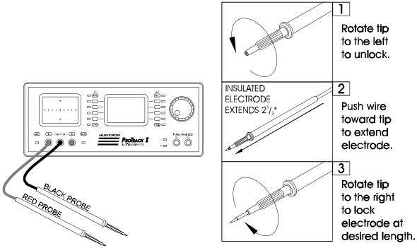
Figure 4-1. ProTrack With Test Probe Leads And Probe Adjustment.
