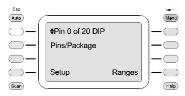
Figure 7-11. Scanner Options Screen With Manual Pin Scan Selected.
