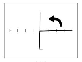
PNP NPN Figure 5-35. Testing Transistors With The Pulse Generator - DC Mode.
