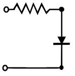
Figure 5-13. Defective Diode Model With A Small Series Resistor.
