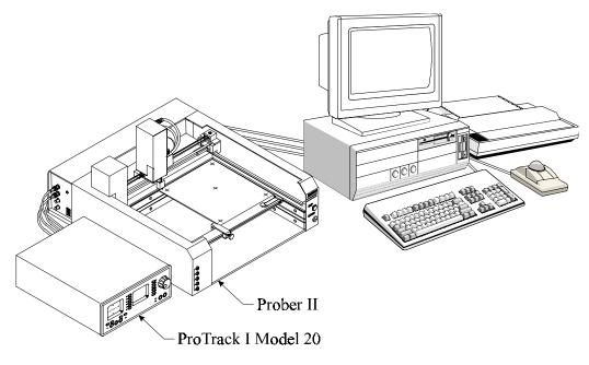
Figure 1-3. ProTrack With Prober II And PC.
