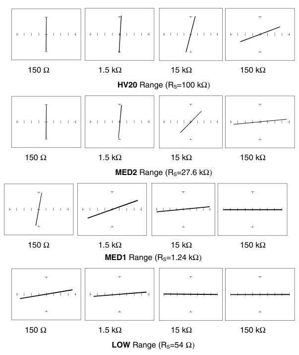
Figure 4-4. Signatures Of Different Resistors In Factory Range Group.
