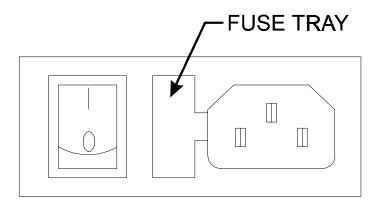
Figure 1-1. Power Entry Module With Fuse Tray.
