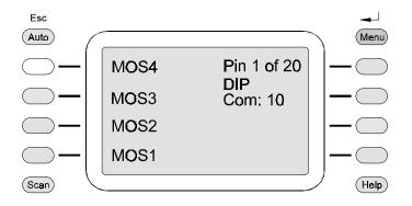
Figure 7-13. Scanner Auto Scan/Compare Pins Screen.
