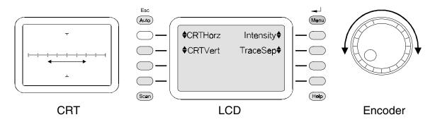
Figure 2-10. ProTrack CRT Horizontal Trace Adjustment.
