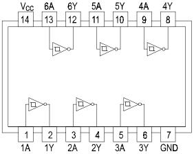
Figure 6-7. 74HC14 Block Diagram.
