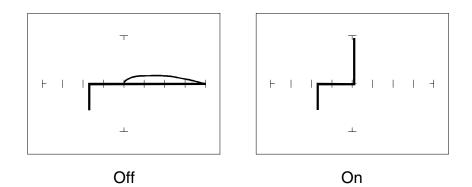
Figure 5-44. Signatures Of An Optocoupler - 4N33 Type MED1 (Factory Group)
