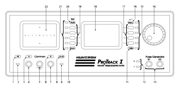
Figure 2-2. ProTrack Front Panel With Callouts.
