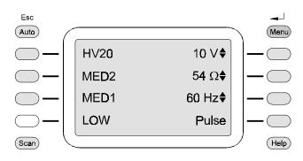
Figure 4-2. ProTrack Main Menu Screen With Factory Defaults.
