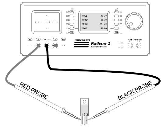
Figure 5-27. ProTrack With Probes To An Unmarked Transistor.
