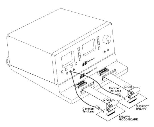
Figure 7-6. ProTrack Scanner Connected To In-Circuit DIP ICs.
