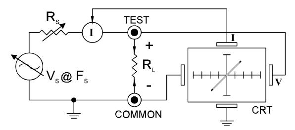
Figure 4-8. ProTrack Tracker Core Circuit Block Diagram With A Resistor.
