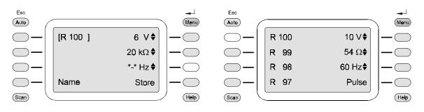
Figure 3-17. User Range With Frequency = \*-\* (Undefined).
