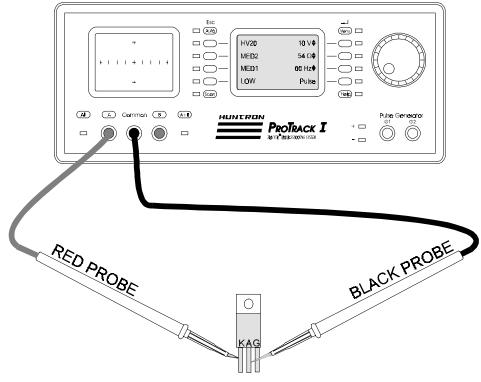
Figure 5-47. ProTrack With Test Leads To A SCR.
