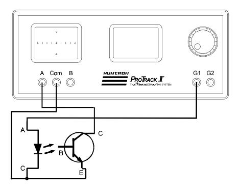
Figure 5-43. Pulse Generator Test Circuit For An Optocoupler.
