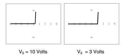
Figure 5-5. Signature Of A 1N914 Type Silicon Diode. LOW Range,  $R_s = 54 \ \Omega$ ,  $F_s = 60 \ Hz$ .
