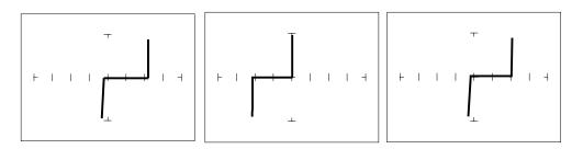
Zener Diode 1N5239B PNP Transistor 2N3906 NPN Transistor PN2222A
