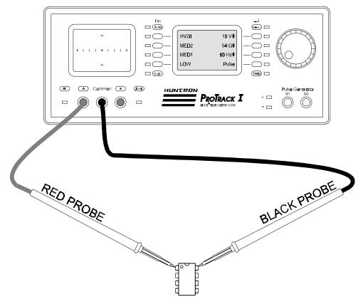
Figure 6-14. ProTrack With Test Leads To An Op Amp.
