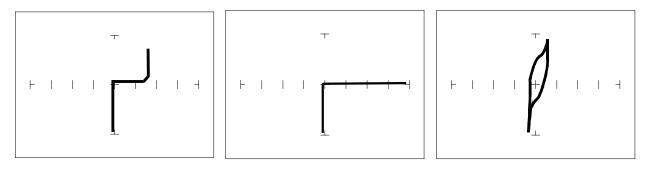
Pin 1 input - TTL3 range Pin 2 output - TTL3 range Pin 14 power - TTL1 range Figure 6-5. Signatures Of A 7404 Hex Inverter. TTL Group
