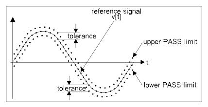
Figure 8-3. ProTrack Compare Tolerance.
