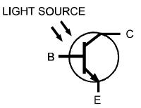
Figure 5-37. Phototransistor Schematic Diagram.
