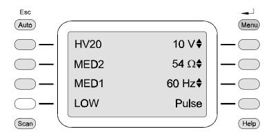
Figure 2-5. ProTrack Main Menu Screen.
