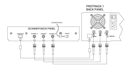
Figure 7-4. ProTrack Scanner And ProTrack Setup.
