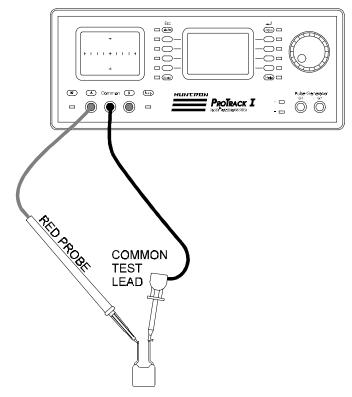
Figure 4-15. ProTrack With Test Probes Connected To A Capacitor.
