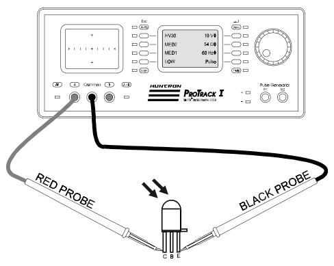
Figure 5-39. ProTrack With Test Probes To A Phototransistor.
