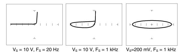
Figure 5-10. Composite Signature - 1N914 Diode And 1  $\mu$ F Capacitor In Parallel. LOW range, R<sub>s</sub> = 54  $\Omega$ .
