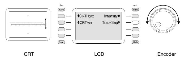
Figure 2-11. ProTrack CRT Trace Separation Adjustment.
