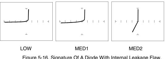
Figure 5-16. Signature Of A Diode With Internal Leakage Flaw. 1N914 Diode With A 10  $k\Omega$  Resistor In Parallel.
