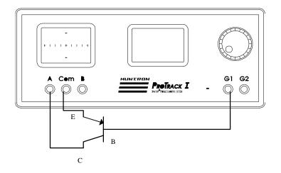
Figure 5-34. Pulse Generator Test Circuit For A PNP Transistor.
