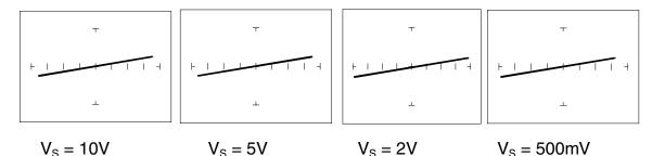
Figure 4-6. Affect Of Varying V<sub>S</sub> On A Resistor Signature. LOW Range,  $R_L = 150 \Omega$
