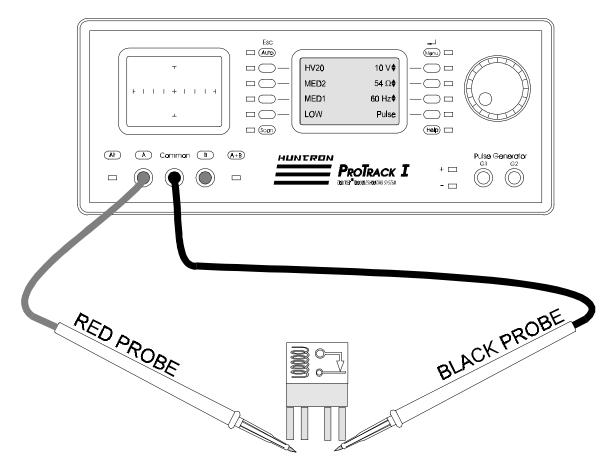
Figure 4-36. ProTrack With Test Leads Connected To Relay's Coil.
