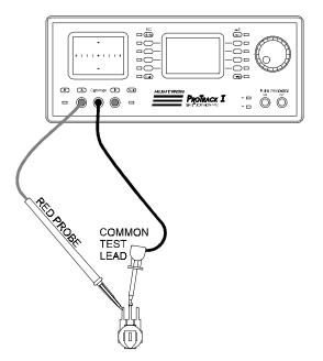
Figure 4-11. Using ProTrack To Test A Potentiometer.
