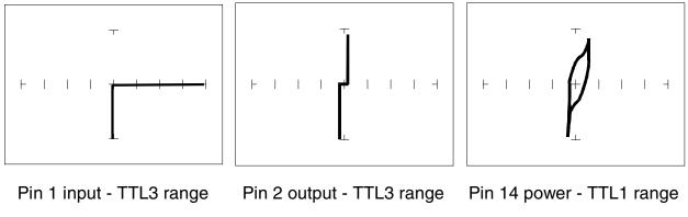
Figure 6-6. Signatures Of A 74LS04 Hex Inverter. TTL Group
