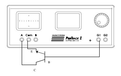
Figure 5-33. Pulse Generator Test Circuit For A NPN Transistor.
