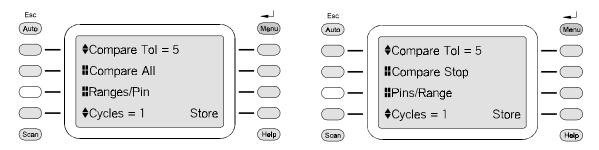
Figure 8-5. Compare Ranges/Pin And Compare Pins/Range Test Order.
