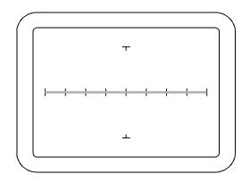
Figure 3-4. ProTrack CRT Display With Open Test Terminals.
