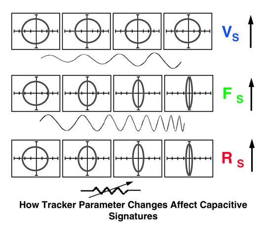
Figure 4-22. Range Parameters Changes And Affects On Capacitive Signatures.
