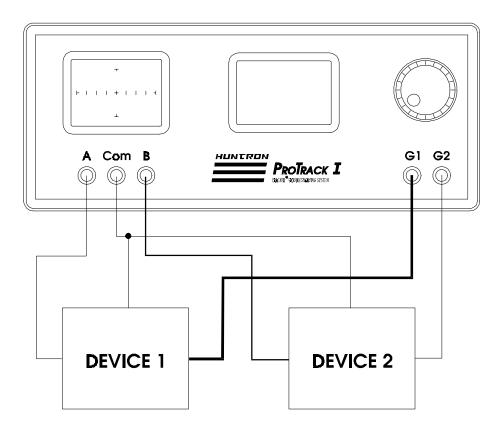
Figure 2-16. Comparison Test With The Pulse Generator.
