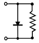
Figure 5-15. Defective Diode Model With An Internal Leakage Resistance.
