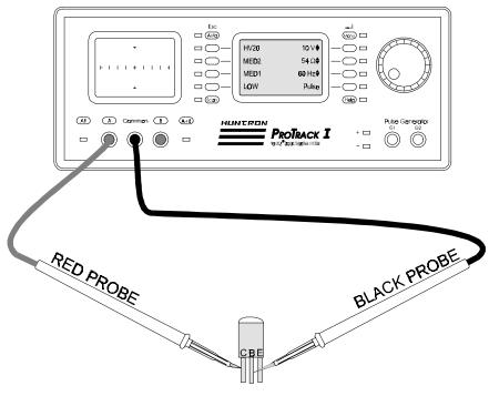
Figure 5-23. ProTrack Connected To The Collector And Base Leads Of A Transistor.
