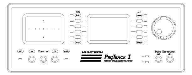
Figure 2-1. ProTrack Front Panel.
