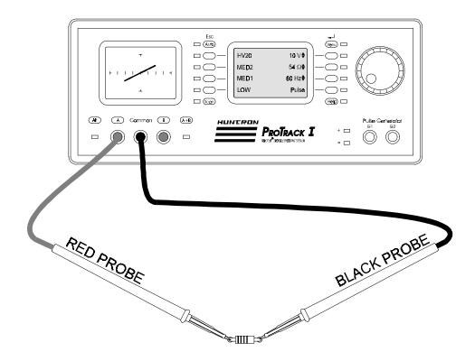
Figure 4-3. ProTrack Connected To A Resistor.
