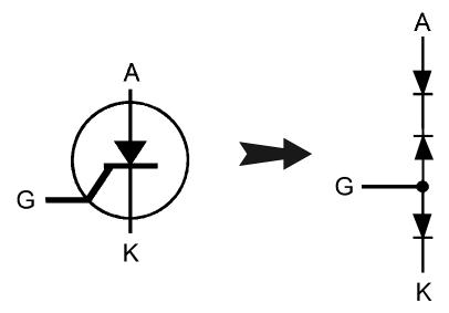
Figure 5-45. Diagram Of A Silicon Controlled Rectifier.
