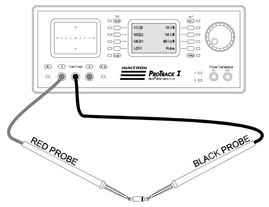
Figure 5-4. ProTrack With Probes To A Diode.
