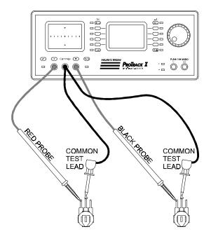
Figure 4-12. Using ProTrack To Compare Two Potentiometers.
