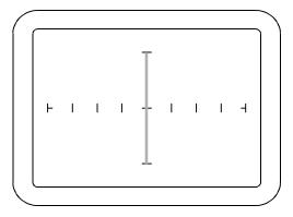
Figure 3-6. ProTrack CRT Display With Short Circuit Signature.
