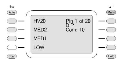
Figure 8-8. Scan/Compare Pin Scan Screen.
