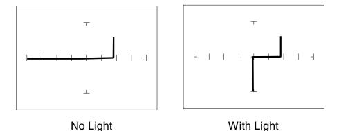
Figure 5-40. Signatures Of A NPN Phototransistor - MRD3056 Type. MED1 (Factory Group), C-E Junction
