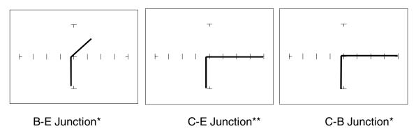
Figure 5-32. Signature Of A Darlington Transistor, TIP112 NPN Type. MED2 Range (Factory Default) Base To Common\*, Emitter To Common\*\*
