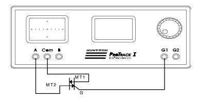
Figure 5-52. Pulse Generator Test Circuit For A TRIAC.
