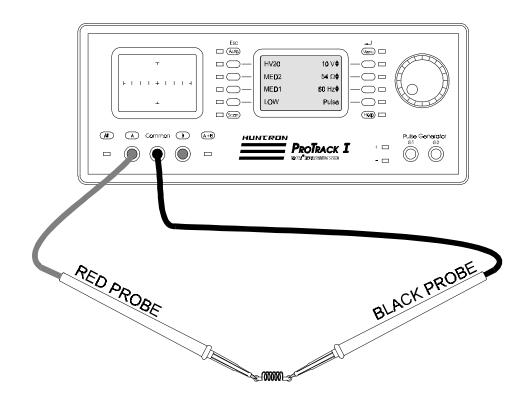
Figure 4-26. ProTrack With Probes To An Inductor.
