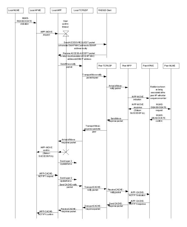
Figure 14—STA reassociation with caching enabled (cache miss)
