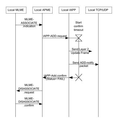
Figure 11—STA association—failure
