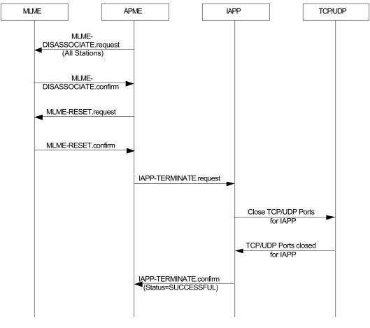
Figure 6—Termination of the IAPP protocol
