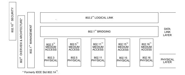
This family of standards deals with the Physical and Data Link layers as defined by the International Organization for Standardization (ISO) Open Systems Interconnection (OSI) Basic Reference Model (ISO/ IEC 7498-1: 1994). The access standards define five types of medium access technologies and associated physical media, each appropriate for particular applications or system objectives. Some access standards have been withdrawn and other types are under investigation.
