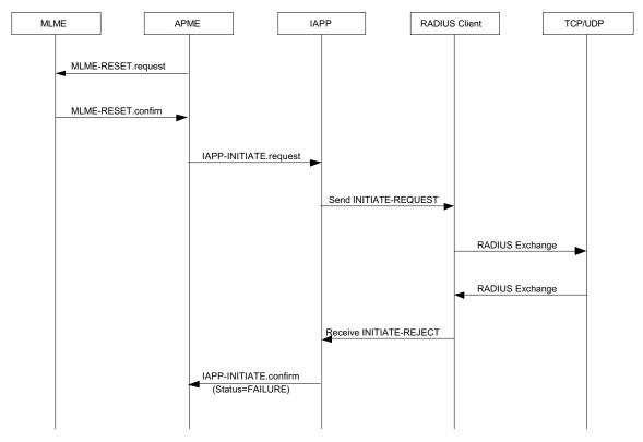
Figure 4—Failed initiation of the IAPP protocol
