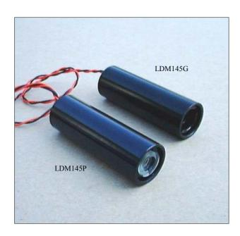
The MaxiBrite Compact laser is a self-contained OEM laser diode module emitting a wavelength of close to 633nm. It has the highest visibility of any of the red laser diodes and can be seen in most daylight conditions.
