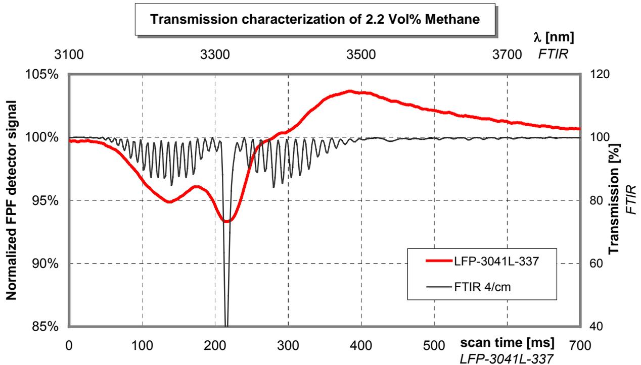
Fig 31: Measurement example for the continuous scan mode with dynamic filter tuning (Methane)
