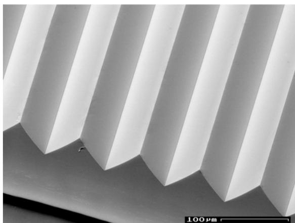
Fig 17: Micro groove (2-channel)
