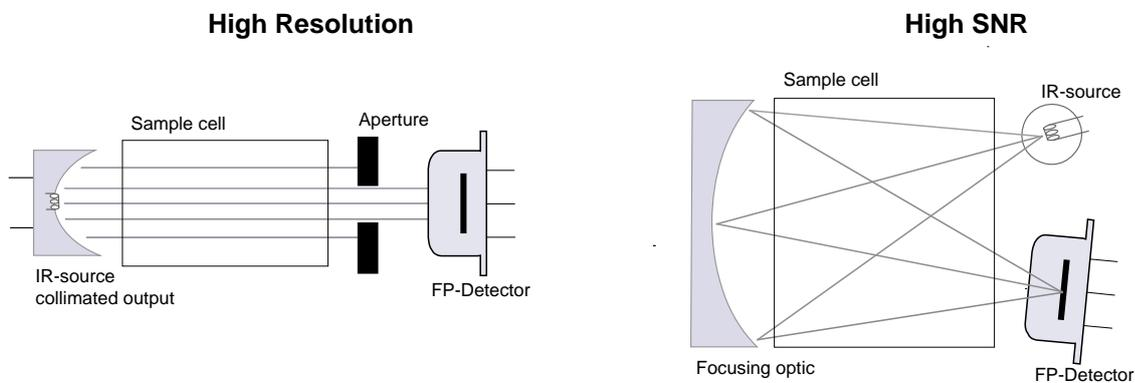
Fig 22: Possible optimizations for the optical design of a microspectrometer with FPF detector **left set up:** corresponds with an illumination by a parallel beam; **right set up:** corresponds with a high angle of incidence (AOI)
