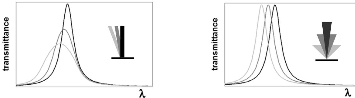
Fig 21: Influence of angle shift and divergence angle on bandwidth and peak transmittance of a FPF
