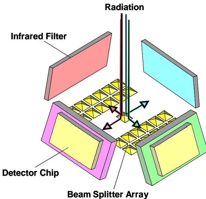
Fig 15: Principle of reflective beamsplittering
