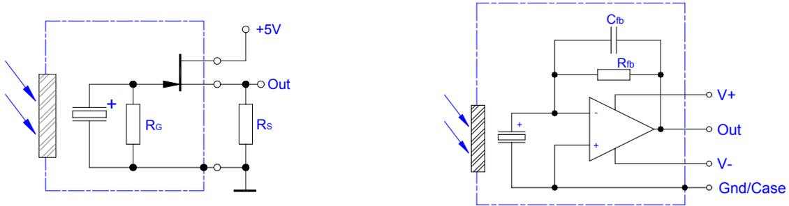
Fig 12: Voltage mode operation (left) and current mode operation (right) of a pyroelectric detector
