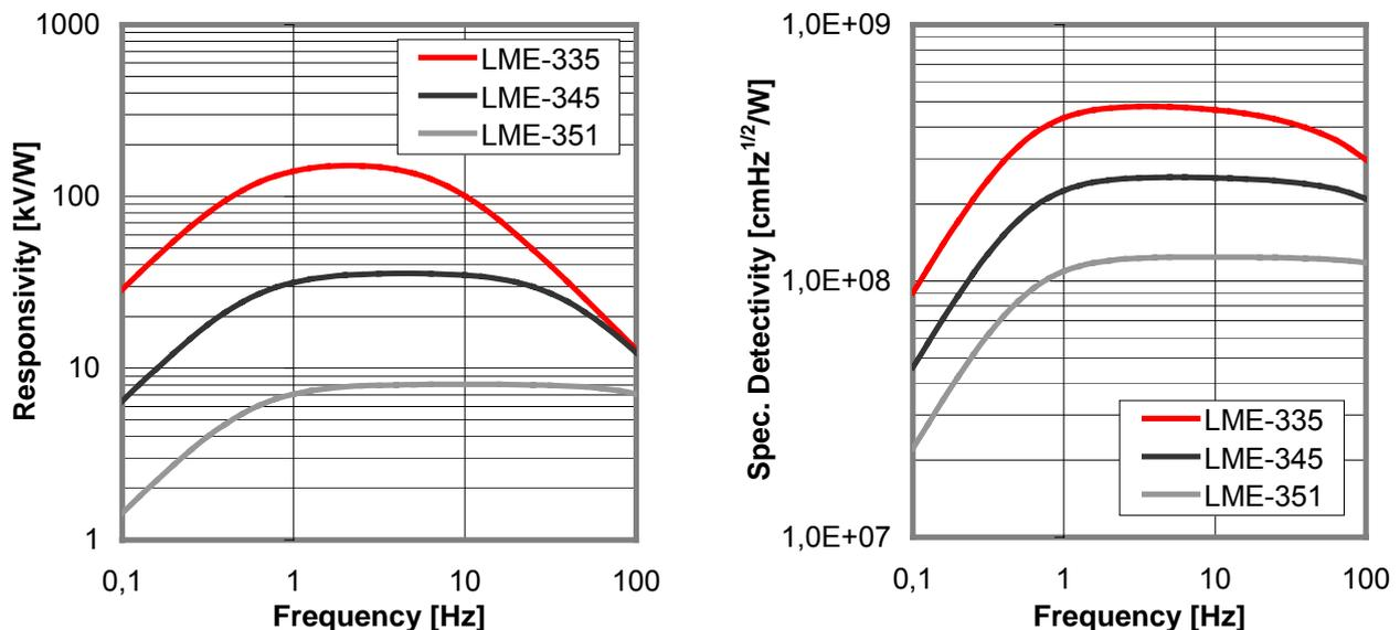
Fig 7: Frequency response of responsivity (signal) and specific detectivity (signal-to-noise ratio) as a function of the feedback resistor; LME-335 (100 GOhm), LME-345 (24 GOhm), LME-351 (5 GOhm)
