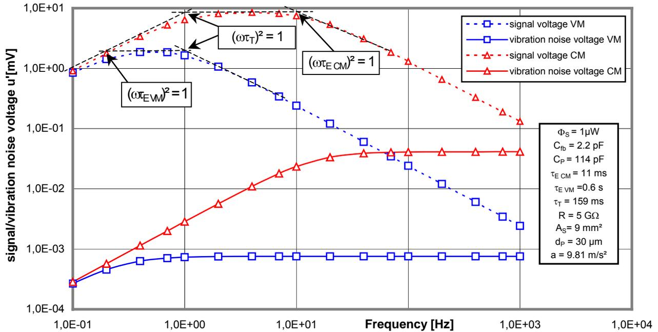
Fig 13: Comparison of the signal voltage  $u'_s$  and of the vibration interference voltage  $u'_{vib\ z}$  (longitudinal effect) in voltage mode and current mode
