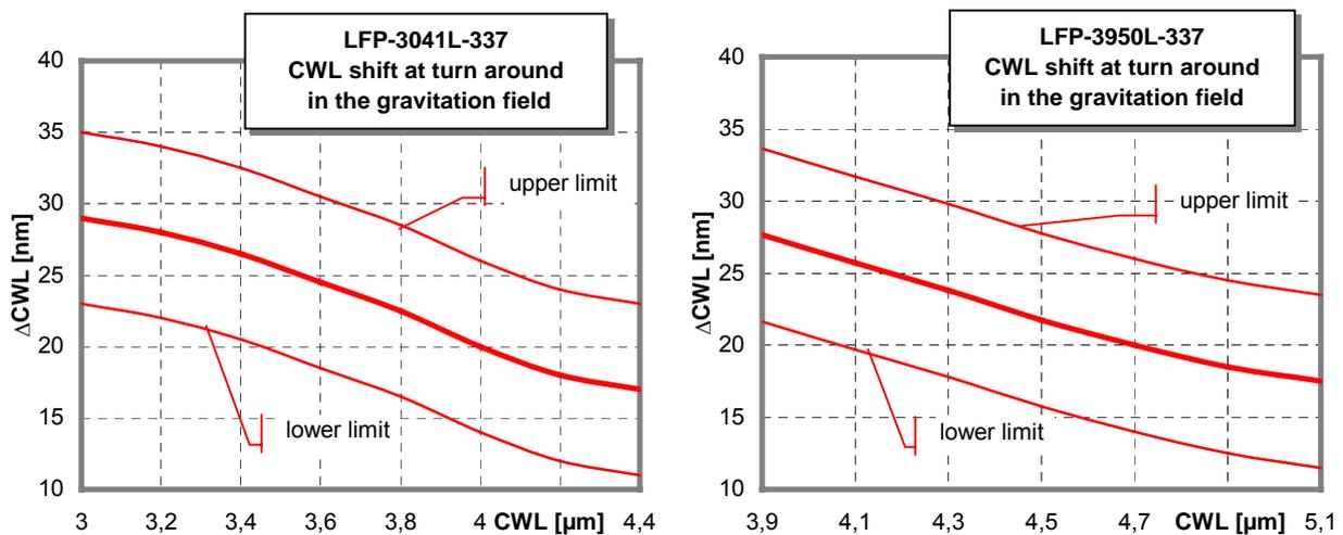
Fig 27: Position dependency of the CWL, typical values and tolerance zones of LFP-3041L-337 (left) und LFP-3950L-337 (right)
