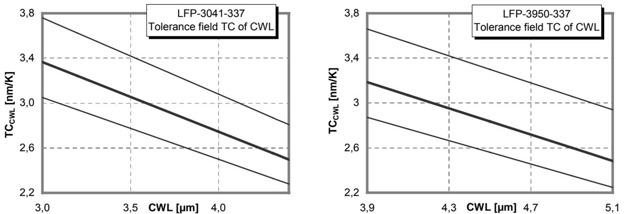
Fig 29: Temperature coefficients of the CWL, typical values and tolerances for LFP-3041L-337 (left) and FP-3950L-337 (right)
