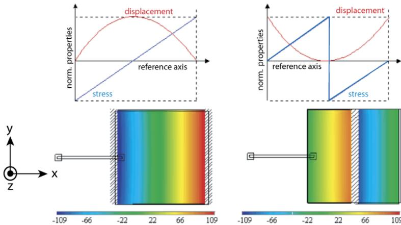
Fig 8: Stress distribution on a double-sided (left), and center (right) clamped pyroelectric detector chip ( $3 \times 3 \times 0.03$ ) mm<sup>3</sup> with acceleration in the X direction
