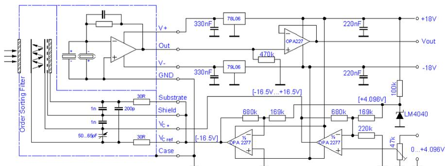
Fig 26: Example of circuitry for detector and filter operation ( $\pm 18$  V bipolar supply)
