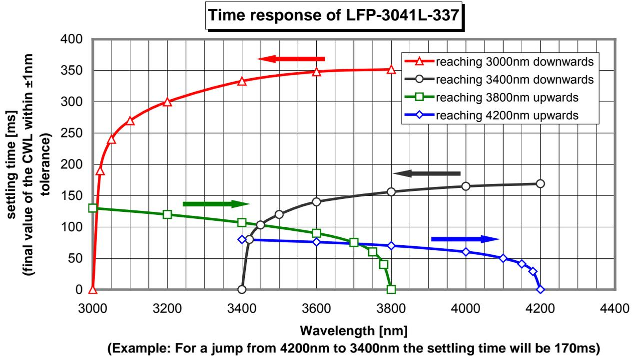
Fig 28: Transient response for LFP-3041L-337, typical values
