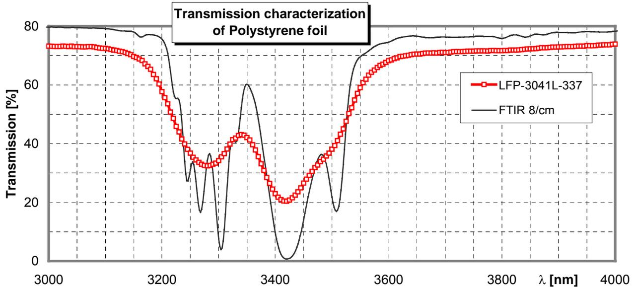
Fig 30: Measurement example for the step scan mode (Polystyrene foil) LFP-3041L-337: spectral resolution  $R=65$ ;  $SNR \approx 1000:1$ ; 100 data points; acquisition time 10 s
