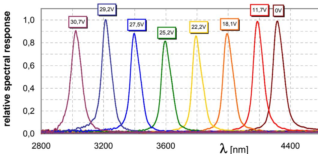
Fig 24: Relative spectral response of a FPF detector LFP-3041L-337 at several tuning voltages
