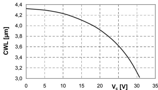
Fig 25: Typical steady-state control characteristic for LFP-3041L-337
