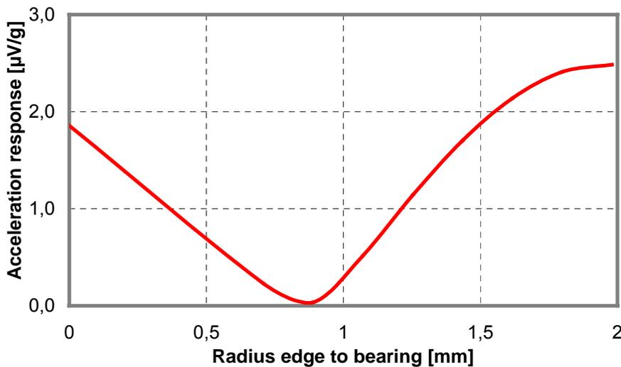
Fig 11: Acceleration response of the chip shown in figure 10 as a function of the mounting point position
