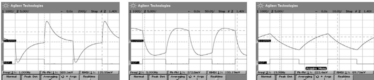
Fig 4: LME-335 Current mode at 1Hz, 5 Hz and 20 Hz, thermal time constant 150 ms, electrical time constant 20 ms
