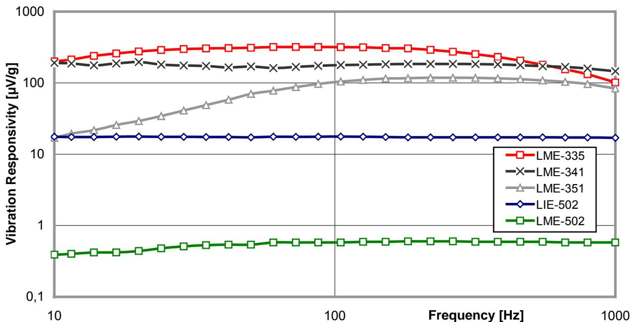
Fig 14: Test results of microphonic effect
