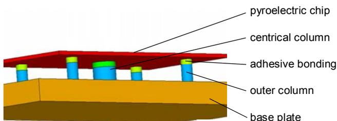
Fig 9: Model of the assembly of chip holder and pyroelectric chip
