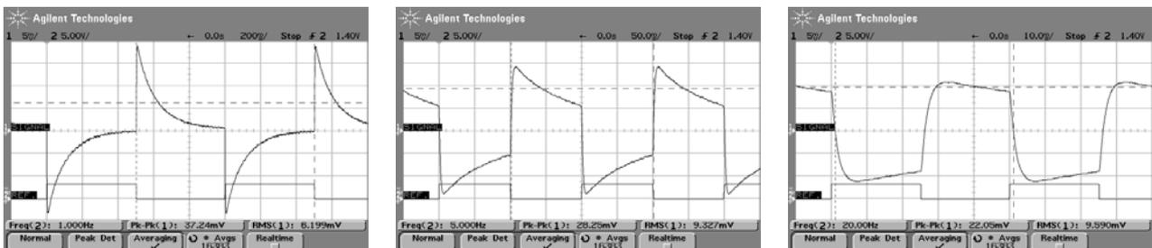
Fig 6: LME-351 Current mode at 1 Hz, 5 Hz and 20 Hz, thermal time constant 150 ms, electrical time constant 1 ms
