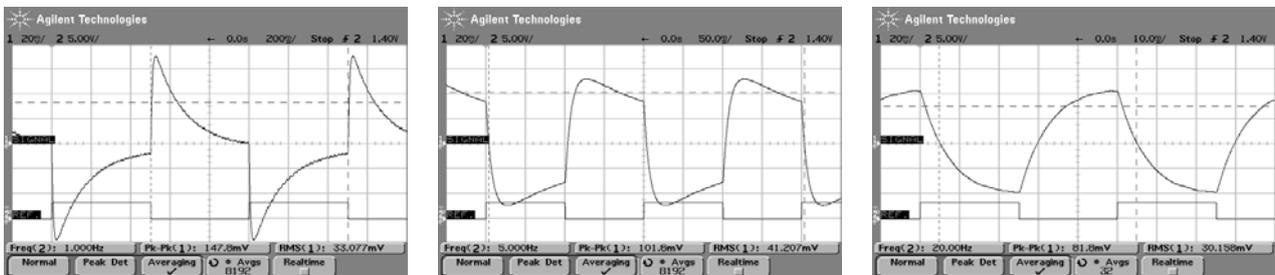
Fig 5: LME-341 Current mode at 1 Hz, 5 Hz and 20 Hz, thermal time constant 150 ms, electrical time constant 5 ms
