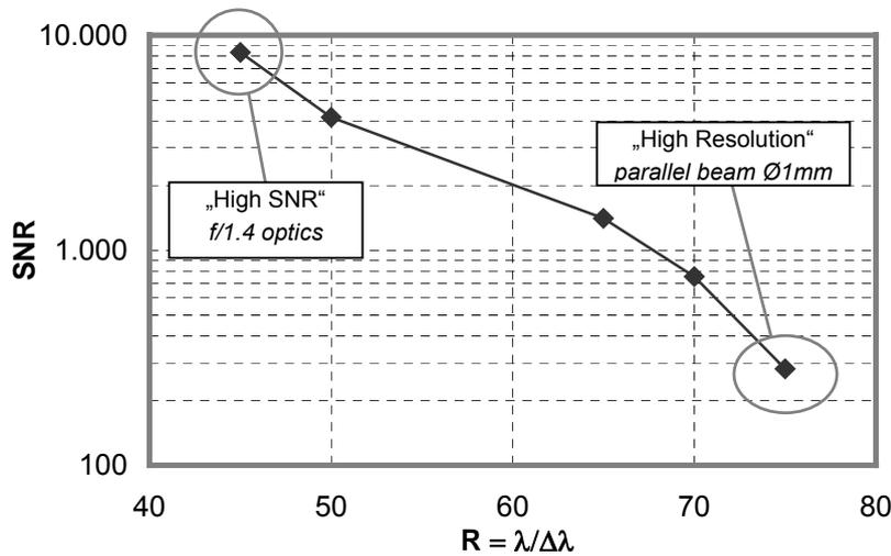
Fig 23: Measurements of the SNR vs. spectral resolution LFP-3041-337 with a modulated IR source at Hz, **left end point:** Illumination at high angle of incidence (AOI) using f/1.4 optics **right end point:** Illumination with a parallel beam  $\varnothing$  1 mm
