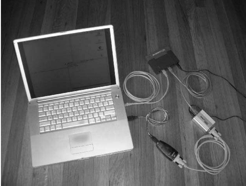
FIGURE 11-11: Full end-to-end test using the SitePlayer Telnet System box
