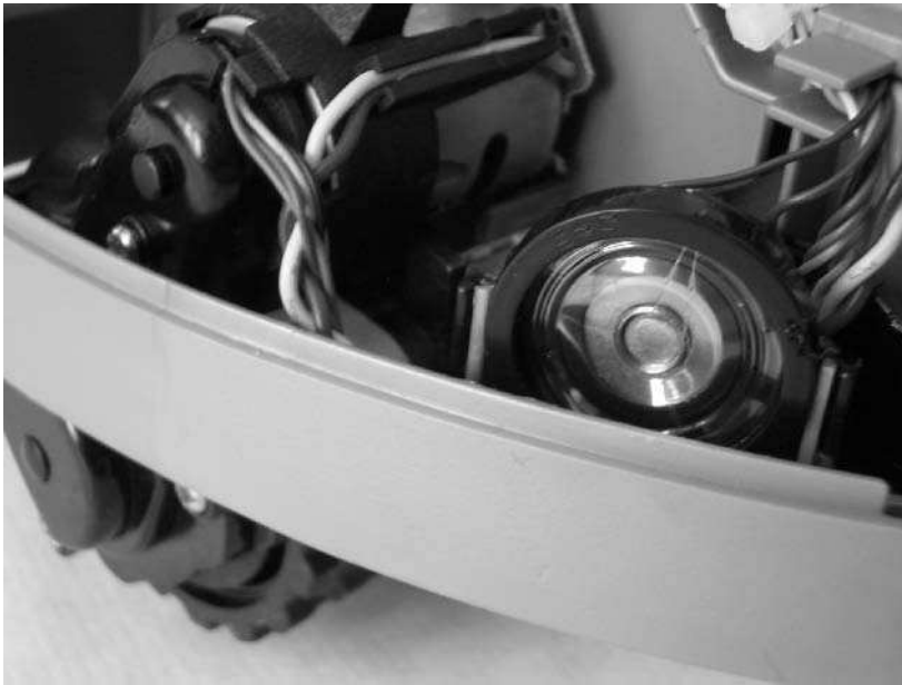
FIGURE 8-2: Piezo beeper inside Roomba
