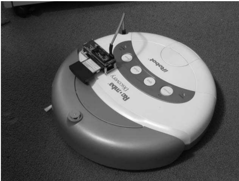
FIGURE 16-3: Tiny Wi-Fi Linux on a Roomba with RoombaNet
