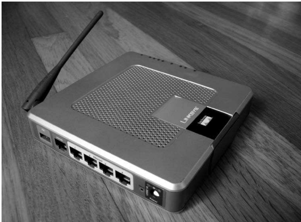
FIGURE 15-1: Linksys WRTSL54GS; note the USB port
