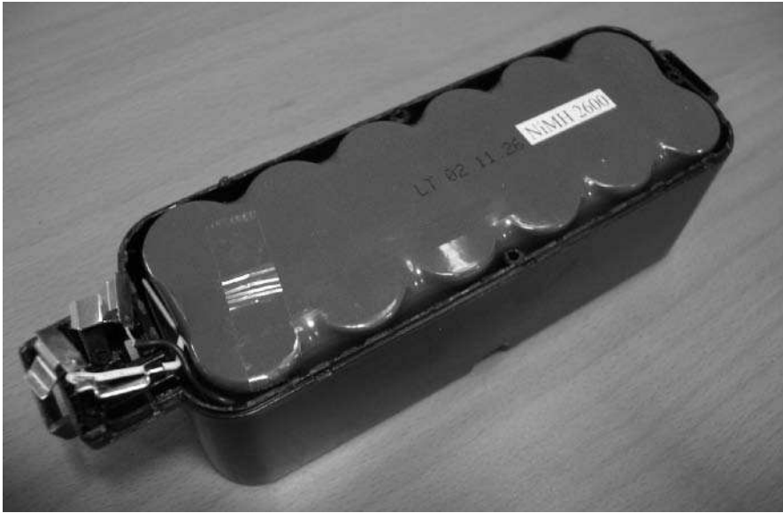
FIGURE 16-14: Battery pack partially apart
