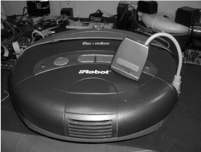
FIGURE 4-9: Bluetooth adapter in a “blue-tooth” enclosure
