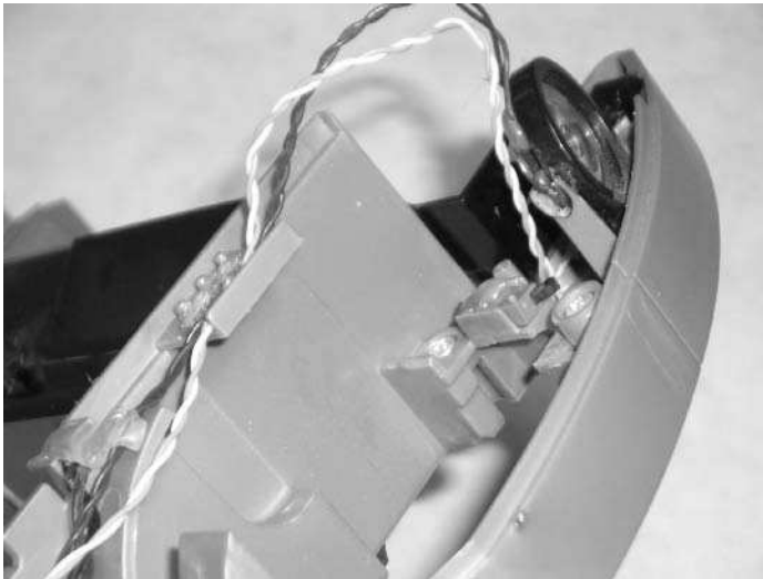
FIGURE 6-6: Wheeldrop sensor, a microswitch
