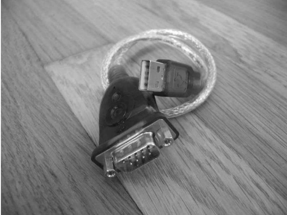
FIGURE 14-9: Generic USB-to-serial adapter, uses PL2303 chip
