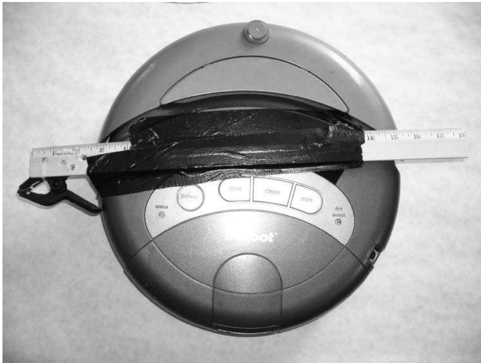
FIGURE 9-6: Ruler and clamp attached to Roomba
