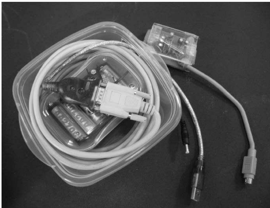
FIGURE 14-15: Serial tether, USB-to-serial adapter, and battery pack, sealed for freshness
