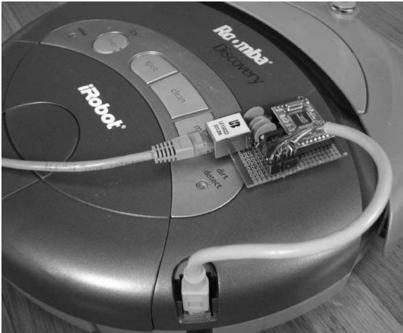
FIGURE 11-13: SitePlayer Telnet Roomba adapter hooked up to Roomba
