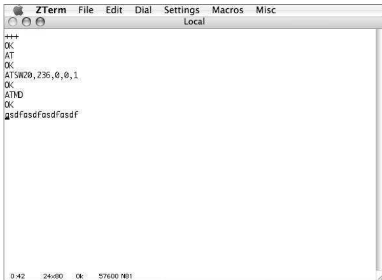
FIGURE 4-16: Changing BlueSMiRF baud rate to Roomba-compatible 57,600 8N1
