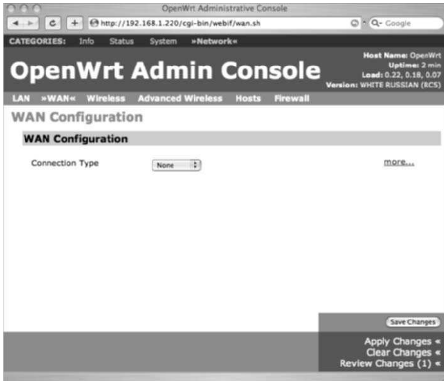
FIGURE 14-7: Disabling the WAN port in OpenWrt
