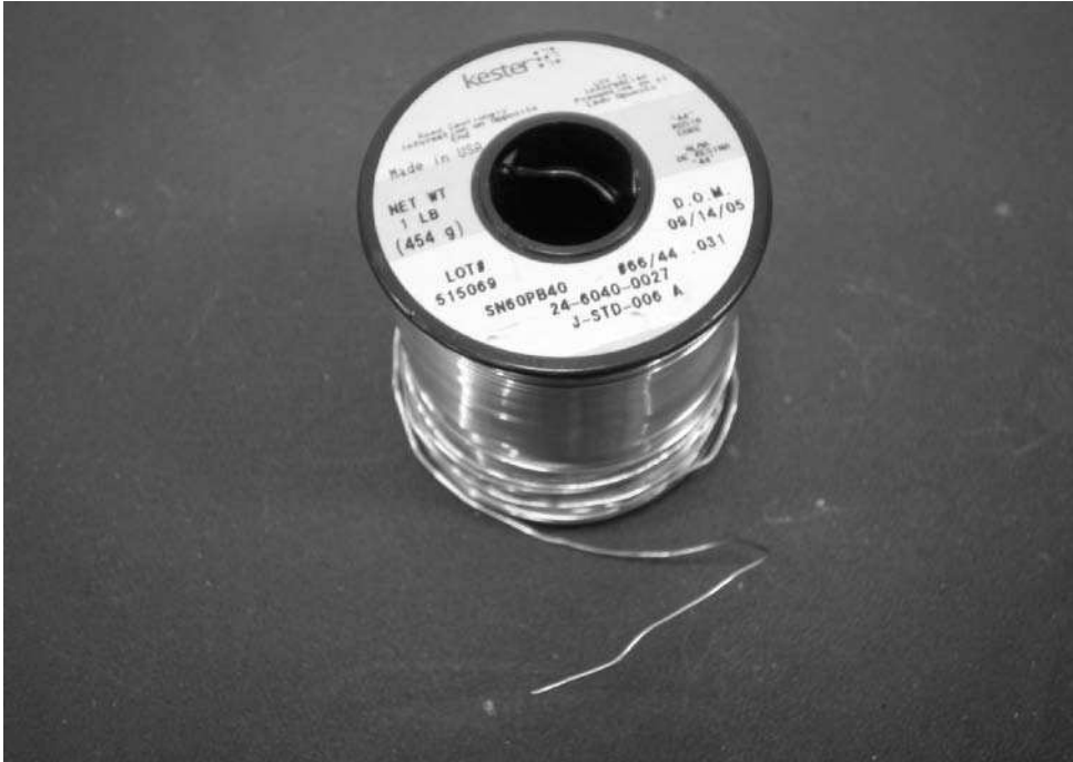
FIGURE A-2: Lead solder, 60/40 .031" rosin flux core
