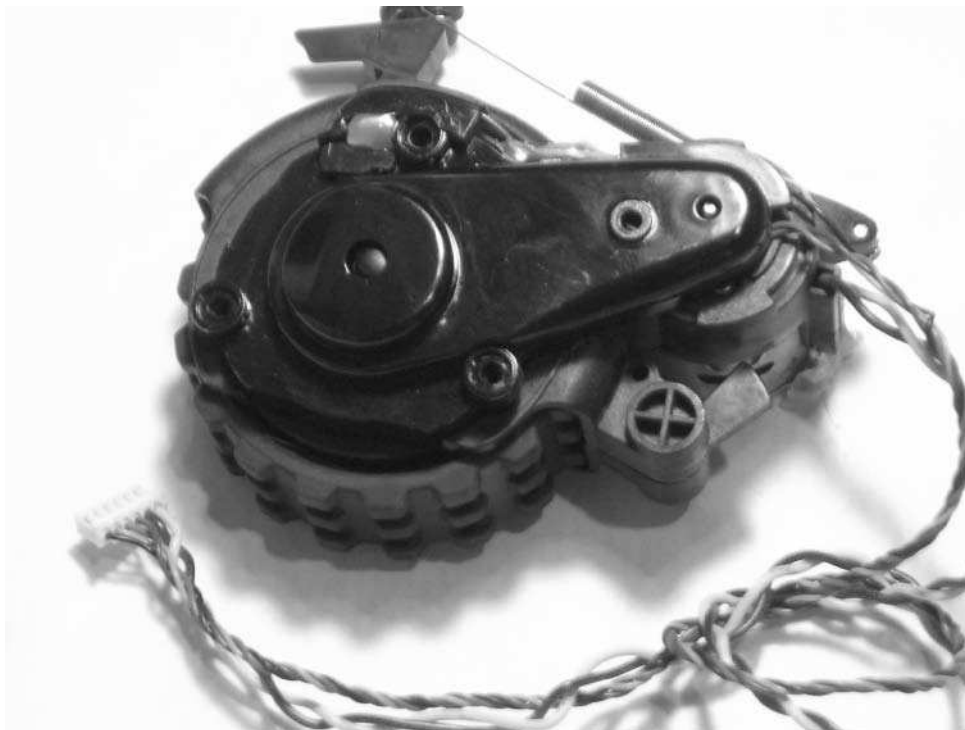
FIGURE 5-1: Roomba drive motor unit
