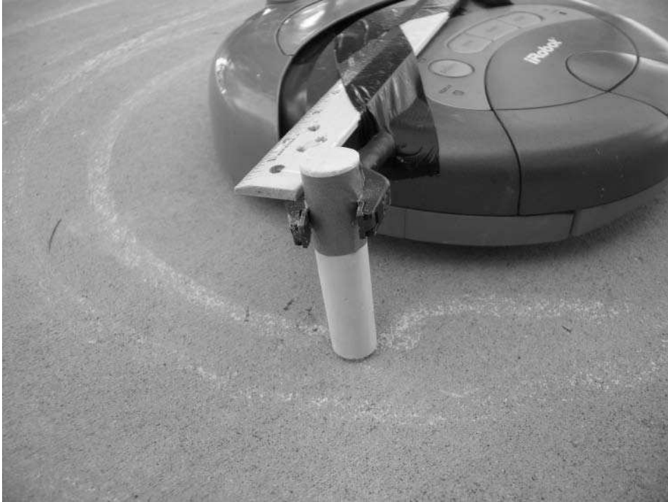
FIGURE 9-7: Ruler and clamp with sidewalk chalk
