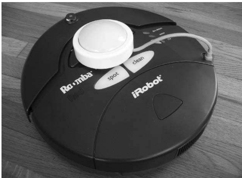
FIGURE 13-27: Arduino Roomba interface inserted into a tap-light for diffuse color
