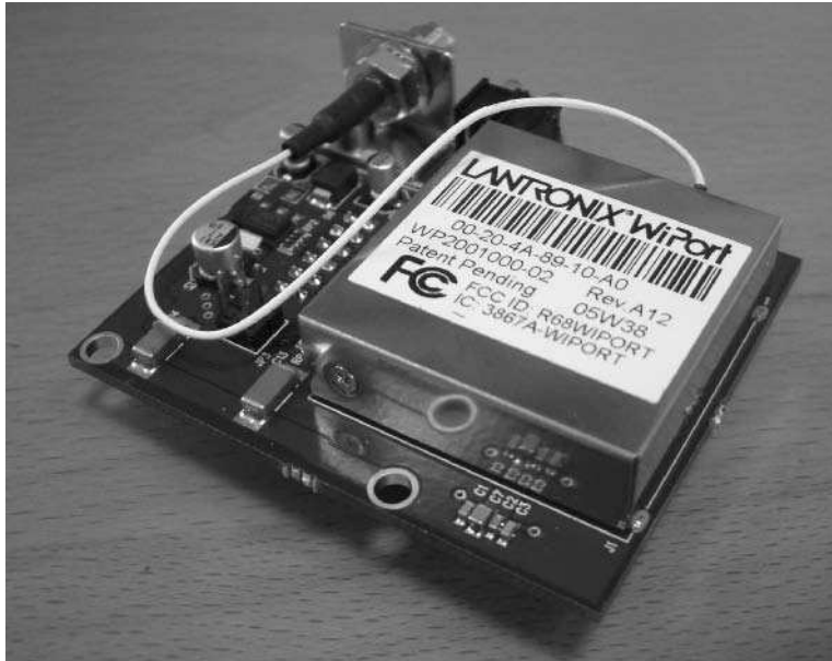
FIGURE 12-2: Lantronix WiMicro board, with WiPort attached
