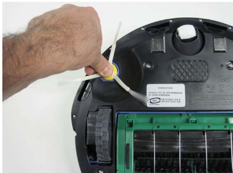
3.2.24 Only once the side brush has been clicked into place properly should you insert the screw into the center of the brush.
