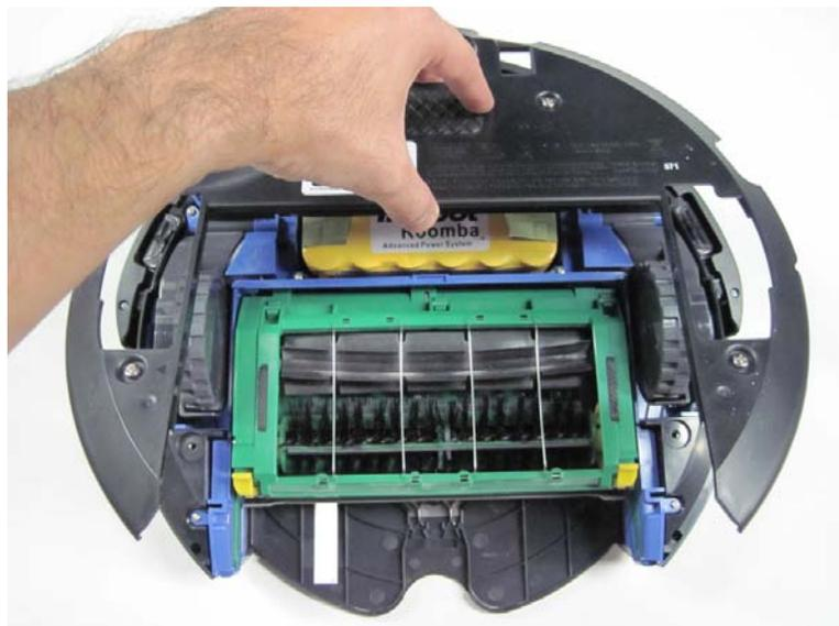
3.2.22 Tighten the bottom cover's four screws until the cover is no longer loose.
