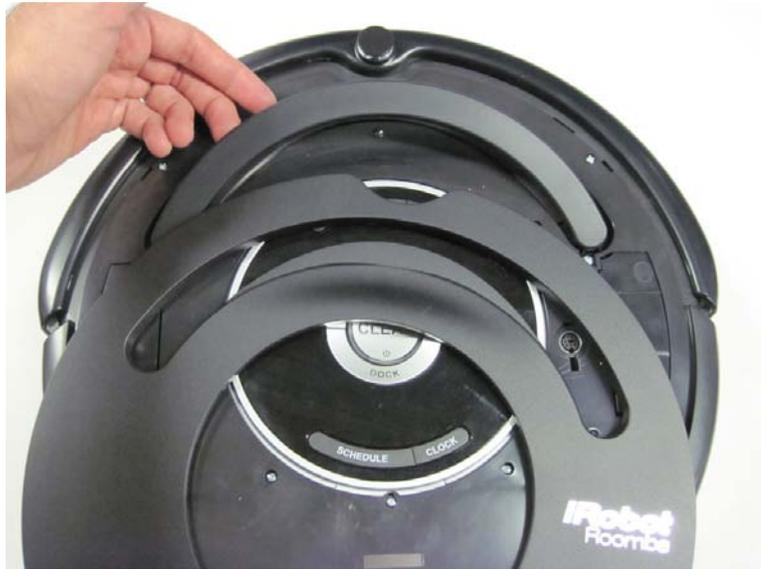
3.2.13 Push the curved tab underneath the handle, while slipping the front edge of the faceplate over the top of the handle.
