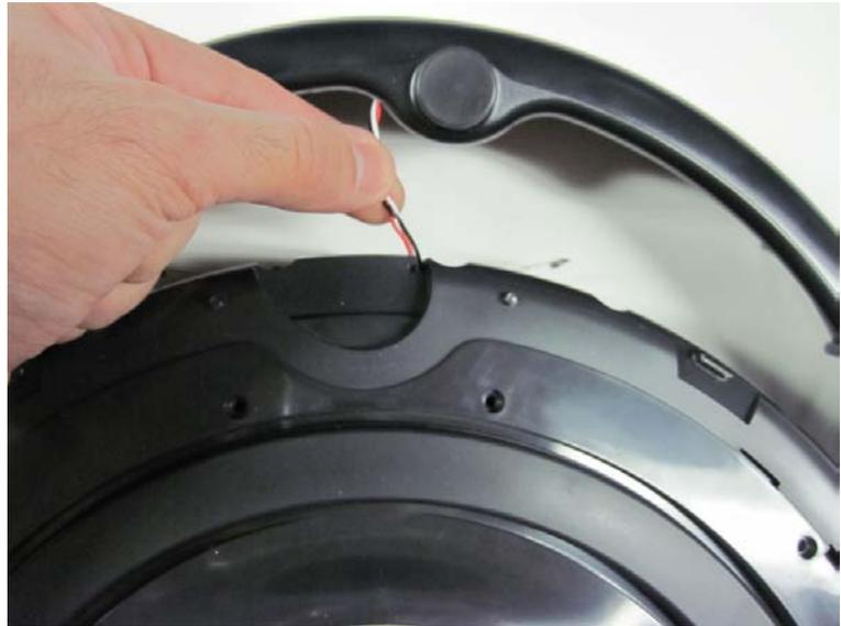
3.2.7 Push the wires into the slot provided on the front end of the top cover. The opening for the slot is small, so you may have to push in one wire at a time.
