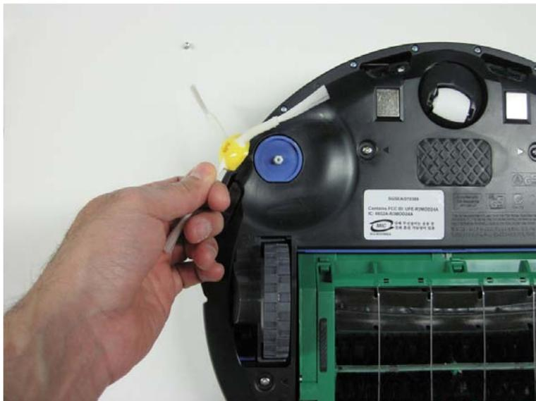
3.1.4 Loosen the four screws holding the bottom cover in place.
