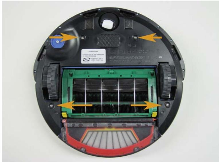
3.1.5 Once the cover is loose, using one of your fingers, hook the bottom cover near the openings for either drive wheel...
