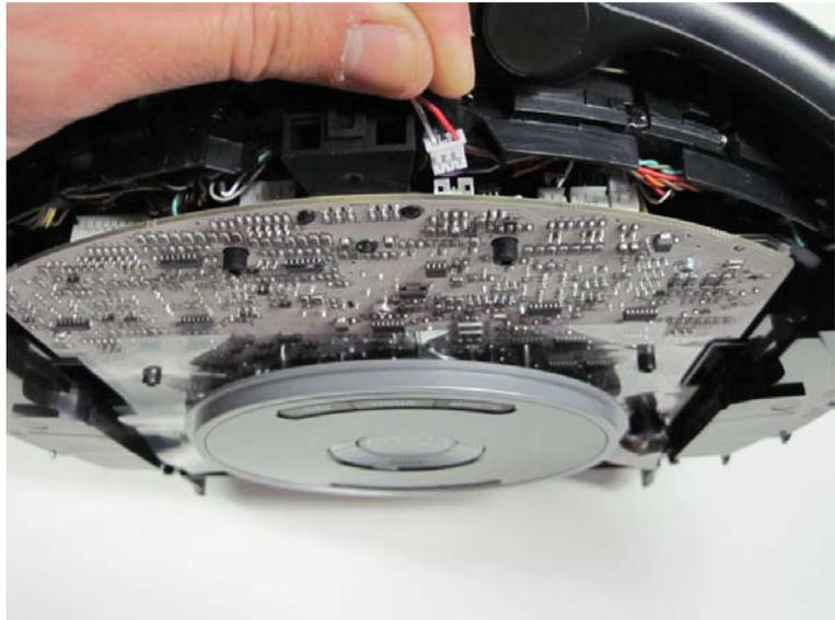
3.2.3 Due to the angle, the connector may be difficult to install all the way without bending backwards the socket on the motherboard. You may want to carefully use a flat-tipped screwdriver (or similar tool) to gently push the connector into place, all the while pushing slightly inwards toward the motherboard to keep the socket from bending.
