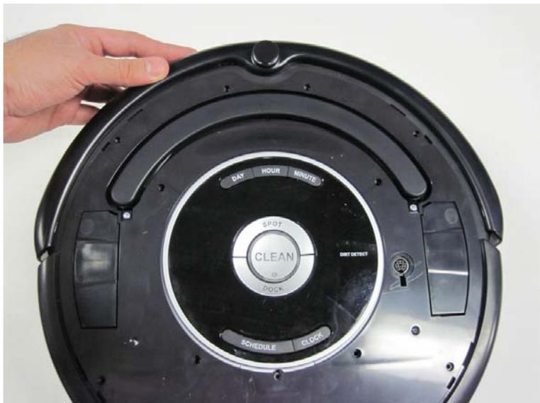
3.2.10 Insert the screw for the top cover, as shown by the orange arrow. It is the only screw of its size (smaller than all the others) that was removed from the top cover.
