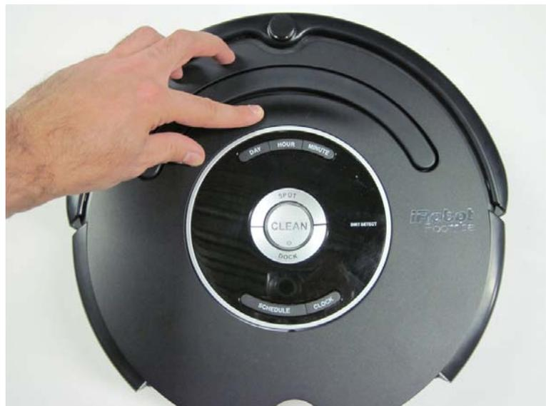
3.2.16 Do the same for the bottom half of the faceplate. Push down firmly on the bottom left and right corners of the faceplate until you hear/feel it click into place, or until the faceplate is flush with the top of the robot.
