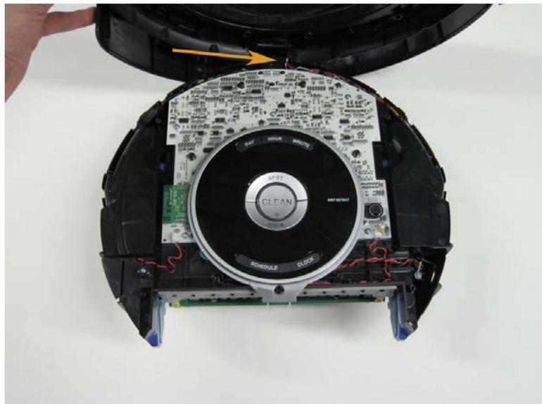
3.1.18 Once the top cover has been removed, the bumper wire remains to be removed.
