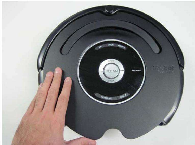
3.2.15 To fasten the front end in place, push down firmly on the top/front part of the faceplate until you feel/hear it click into place, or until the faceplate is flush with the top of the robot.
