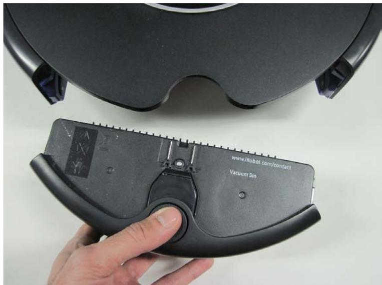
3.1.12 Remove the faceplate from the Roomba. Starting at the bottom where the dustbin goes, lift up the edge of the faceplate, and insert a long screwdriver (or similar tool) into the gap. Then, while holding the Roomba in place, lift the handle end of the screwdriver like a lever to un-clip the faceplate from the Roomba.
