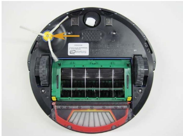
3.1.2 Once the screw is removed, you can grab the side brush by any two of its three brushes and pull up away from the robot.
