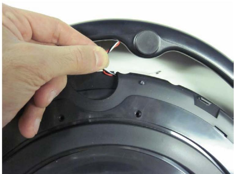
3.2.8 Push the top cover down into place on the frame. Position the wiring for the bumper so that any slack in the wires curls around, following the shape of the groove on the front of the top cover, as shown by the orange arrows.
