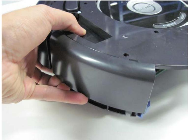
3.1.15 Do this for both sides of the robot, pushing down on the frame with your thumb (orange arrows), and lifting up the bottom edge of the cover with your finger tips (red arrows).
