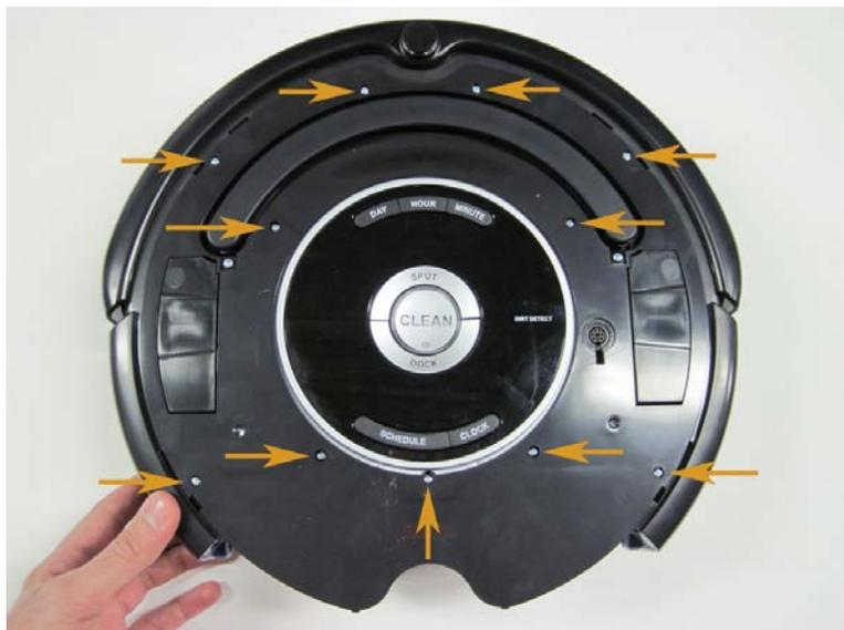
3.1.14 Loosen the top cover from the robot by lifting the edge of the cover up, while pushing down on the main frame with your thumb, as pictured.
