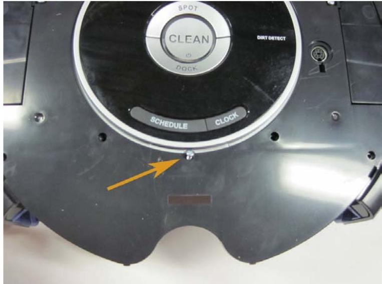
3.2.11 Insert the remaining screws for the top frame cover, as shown by the orange arrows.
