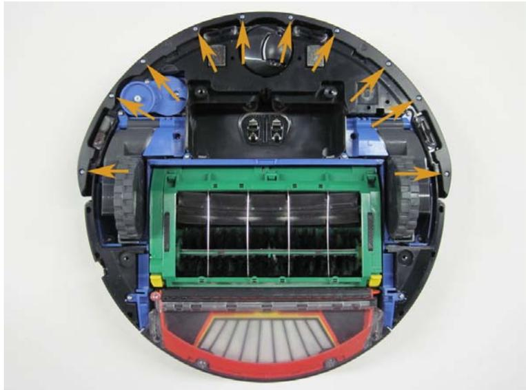
3.1.9 With the screws loose, now remove the bumper's bottom trim piece from the robot.
