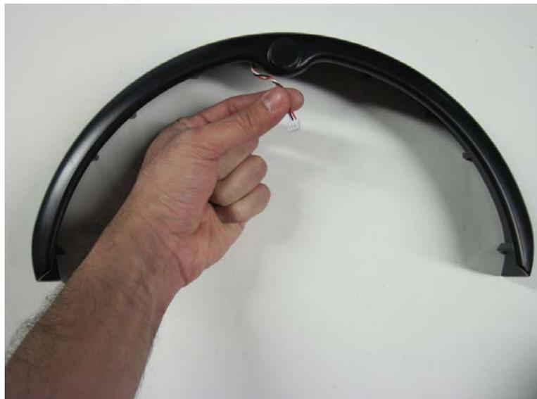
3.2.2 Reinsert the bumper wire connector into its socket.
