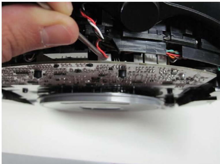
3.2.4 With the bumper wire connected now, leave the bumper loose in front of the main unit.
