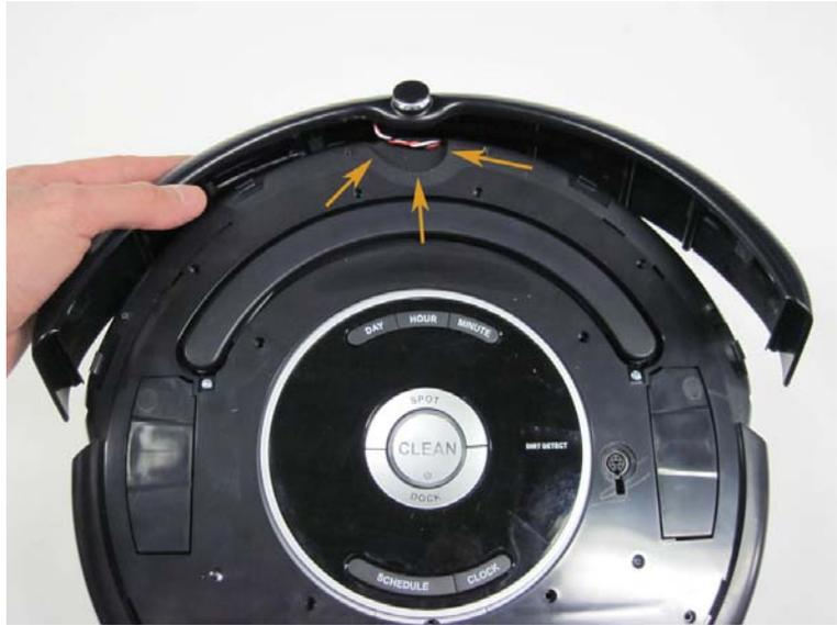
3.2.9 Place the bumper properly on the front of the unit, over the top cover.
