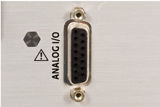
FIGURE 6-6 Analog I/O connector
