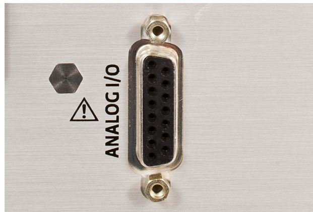
FIGURE 3-14 Analog I/O connector
