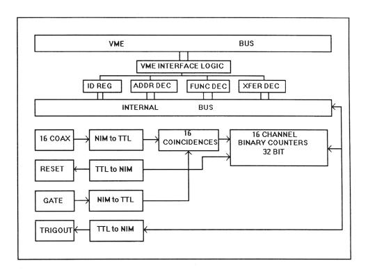
Figure 5: Block Diagram of the 1151 Scaler
