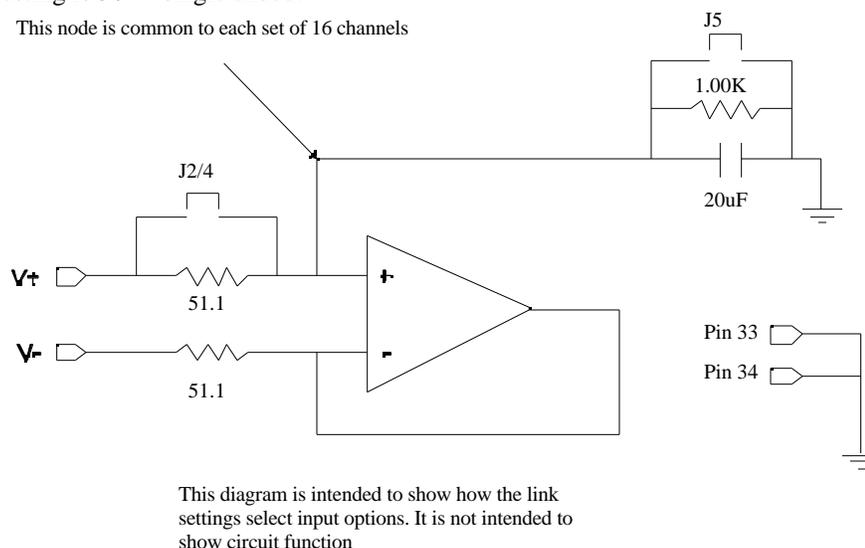
Figure 3-1 Input Circuit
