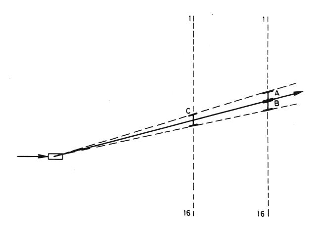
Looking at the figure let's suppose to have two hodoscope planes and that a trigger is required when the two planes are traversed by a particle originated from the target.
