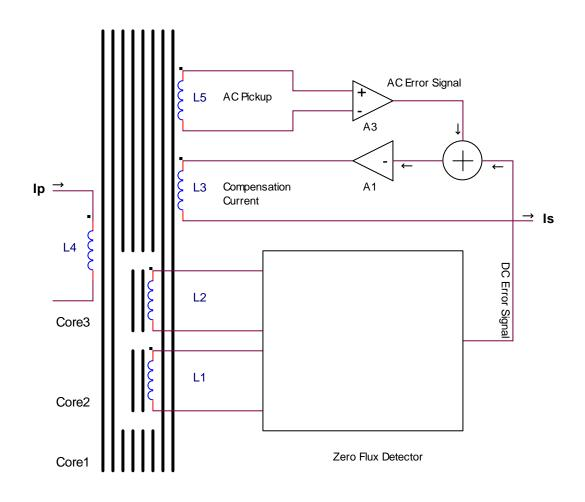
The transducer head core (1) is the basic body structure. The cores (2) and (3) are flux detector cores coupled to the electronics zero flux detector circuitry by means of the coils L1 and L2. L1 and L2 are coupled in parallel or serial, depending of model, with opposite phase to reduce the unwanted flux generated in Core1.
