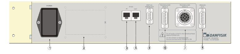
All connectors on the ULTRASTAB SATURN are placed on rear of the unit.
