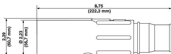
Taper Nose In-line Latching Male Connectors - Crimped
