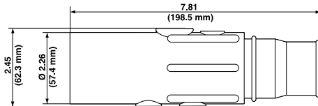
Ball Nose In-line Latching Male Connectors - Crimped
