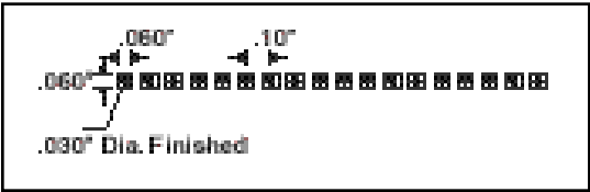
Figure 11: Suggested PCB Footprint
