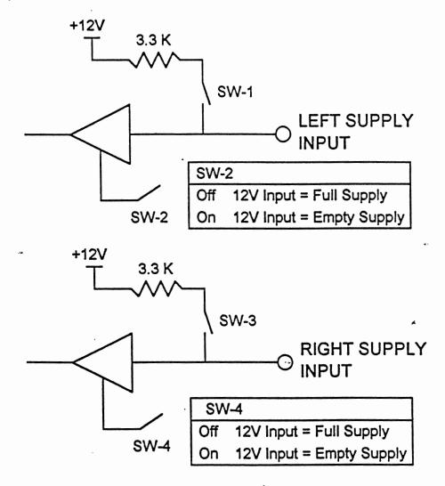
The type of input switch used will determine the switch settings. Use the following examples to determine your configuration.
