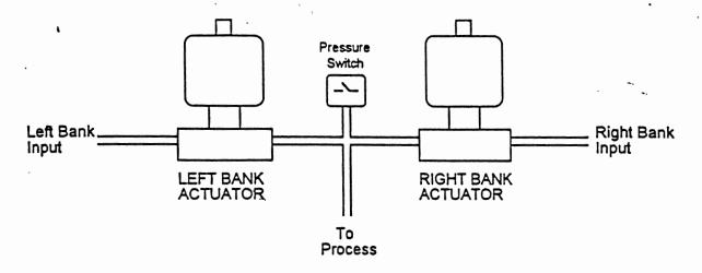
The input signal from this switch is connected to the LEFT INPUT terminal only.
