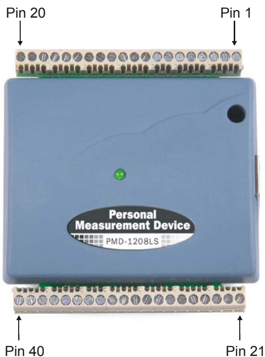
Figure 3-2. PMD-1208LS Screw terminal pin numbers
