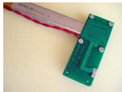
1100-20 mounted for \delta B_y/\delta x correction.
