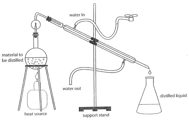
Adjust the apparatus so that all connections are tight.
