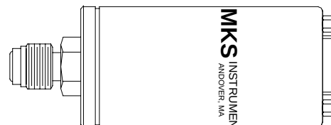
Figure 5: Acceptable Horizontal Mounting Positions
