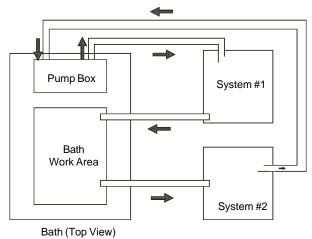
The pump can be used to circulate through two closed loop systems. Connect the shortest practical length of flexible tubing from the PUMP OUTLET to the inlet of external system #1. Connect the outlet of system #1 directly into the bath work area. Connect tubing from the bath work area to the inlet of system #2. Connect the outlet of system #2 to the PUMP INLET.
