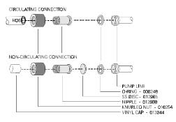
installed using Teflon® tape around the threads.)
