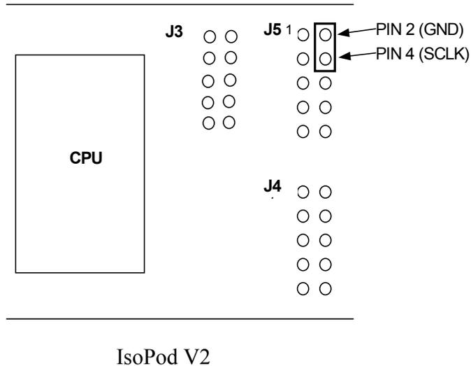
This connects the SCLK/PE4 pin to ground. When the IsoPod detects this condition on reset, it does not perform the autostart search.
