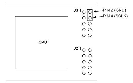
This connects the SCLK/PE4 pin to ground. When the IsoPod detects this condition on reset, it does not perform the autostart search.
