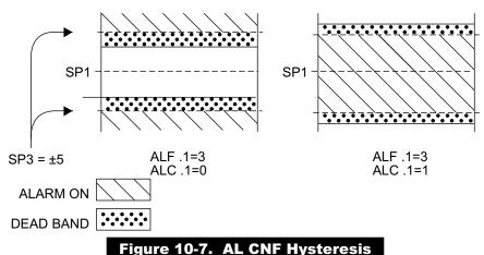
Figure 10-7 Illustrates the Alarm configuration for hysteresis.
