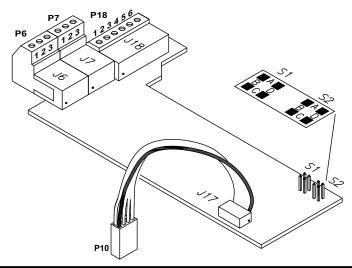
Figure 14-2. 4 Relay Board Jumpers and Plugs.
