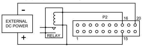
Figure 16-2. Connection of External Power for Setpoint Transistors
