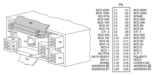
Figure 13-1. BCD 40-Pin Cable Connector (P8)
