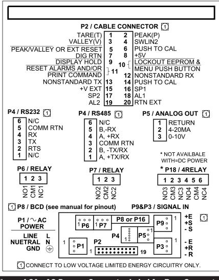
Figure 4-2A. AC Power - Connector Label for Rear Connectors
