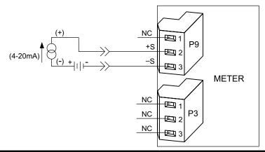
Figure 7-1. Current Input Without Sensor Excitation
