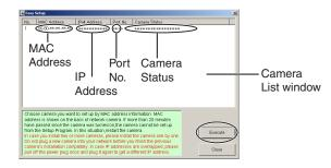
• The MAC Address on the rear side (see page 5 of the Operating Instructions on the CD-ROM.) of the camera shows which camera you select on the camera list window.
