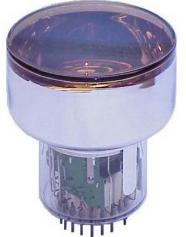
The 83095 600 is a compact, low profile 3" (76mm) head-on PMT designed specifically for gamma camera use but is ideal for a host of general scintillation counting applications. The 83095 600 8-stage design offers excellent energy resolution and long term stability
