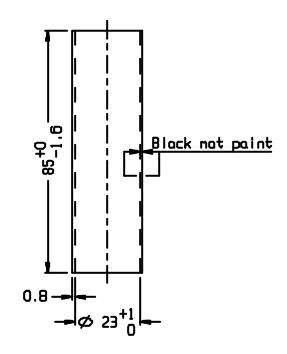
Magnetic shield for fast 3/4" (19mm) tubes Such as XP1911, XP2802, XP1117
