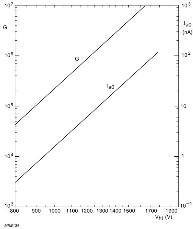
Fig.2.8 Examples of photomultiplier gain and anode dark-current variation as functions of applied voltage
