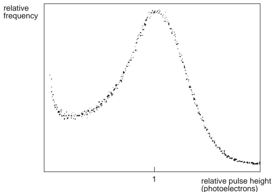
Fig.2.4 Typical single-electron spectrum. Resolution 67% FWHM.
