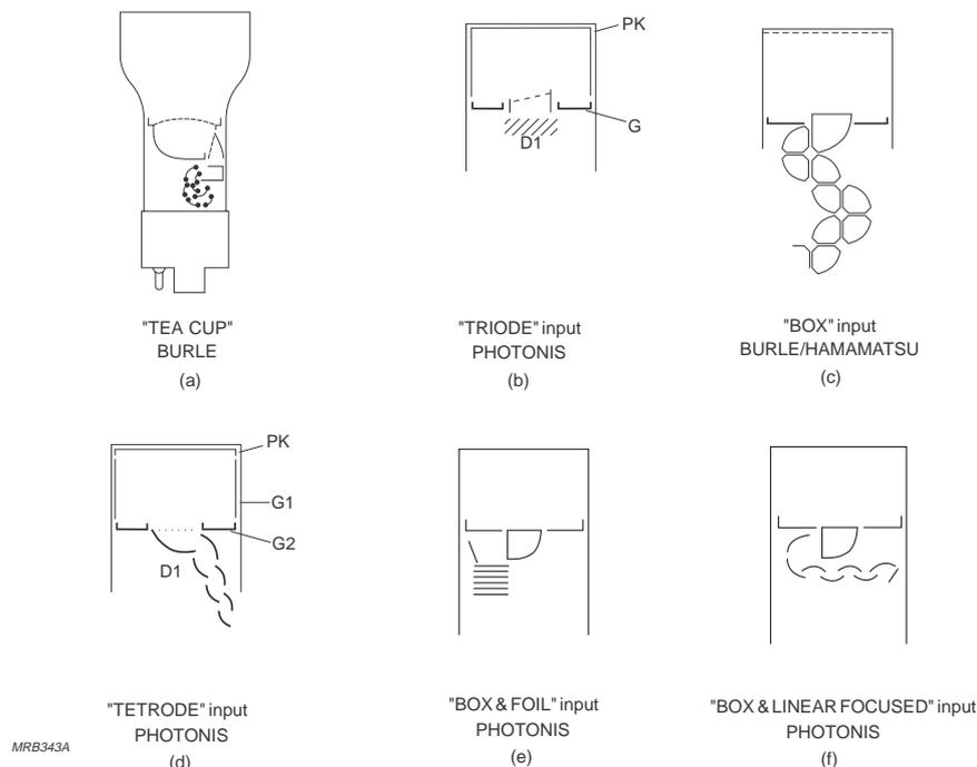
Fig.7.2 Examples of  $\gamma$ -camera tube input systems
