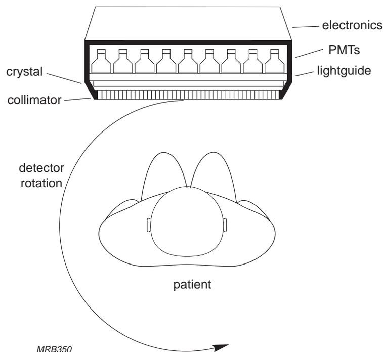
Fig.7.3 Principle of single-photon emission computed tomography (SPECT). The  $\gamma$ -camera head (sometimes 2 or 3) is moved around the patient and acquires projections from several angles. These are back-projected by computer to give transversal slices
