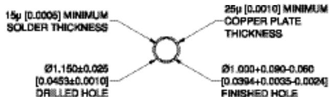
SIZE 20 PRESS-FIT CONTACT HOLE
