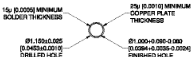
SIZE 22 PRESS-FIT CONTACT HOLE
