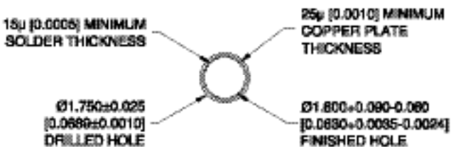
SIZE 16 PRESS-FIT CONTACT HOLE
