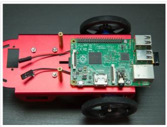
Pi's rear mounting holes (near the USB ports) are directly above the long mounting slot at the back of the chassis. Use the #4-40 machine screws and nuts to screw through the Pi and cardboard to securely hold the Pi in place.
