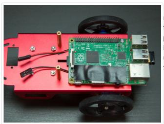
If you aren't using Pi HAT standoffs to hold the motor HAT place a piece of electrical tape across the HDMI connector side of the Pi. This will help prevent the motor HAT from getting pushed down into the connectors and shorting out. If you are using the standoffs you can place them over the front mounting holes of the Pi (not shown).
