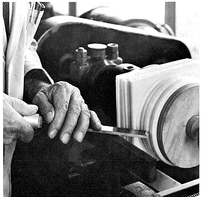
Fig. 4: Circular discs or cylindrical parts are produced on the turner's or wood turner's lathe. The required gripping forces are transmitted by wooden discs.
