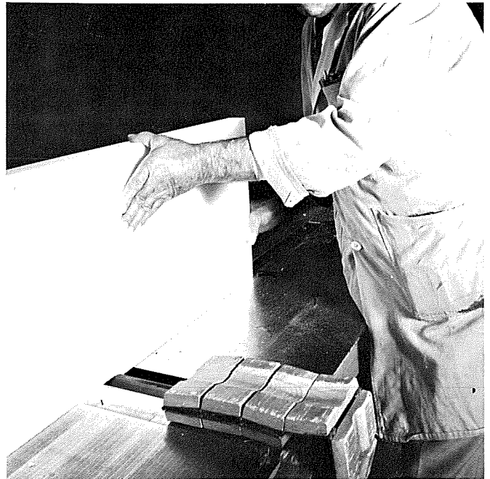
Fig. 2: For planing edges and faces one uses ordinary wood planing machines. Thicknessing machines are also suitable. Since the foam is easily dented, the profile of the draw-in rollers may show on its surface. Therefore, the cutting depth should be chosen with a view to removing such impressions.
