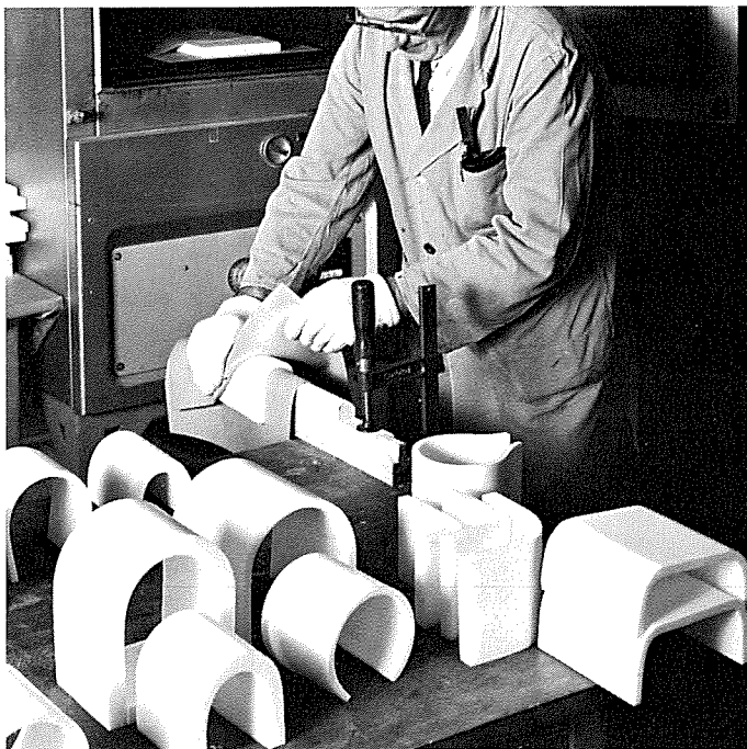
Fig. 11: Curvatures are produced by thermoforming. Due to the high thermoforming temperature of 170 – 190 °C the foam would cool down very quickly after removal from the heating cabinet and cracking would occur. Therefore it is packed between cotton glove cloth or silicone rubber sheets, which prevent fast cooling.
