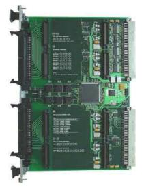
A set of 16-position rotary switches allows easy configuration of VME Short I/O and Memory addresses. Interrupt routing from the IP slots to the VME IRQ's can be done in two ways: programmable by software or selection of predefined sets by a rotary switch.
