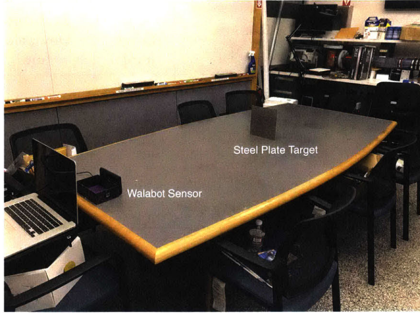
Figure 3-4: Image of test setup for radial testing
