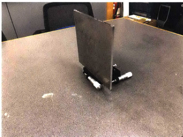
Figure 3-5: Image of steel target on optical stage for resolution test
