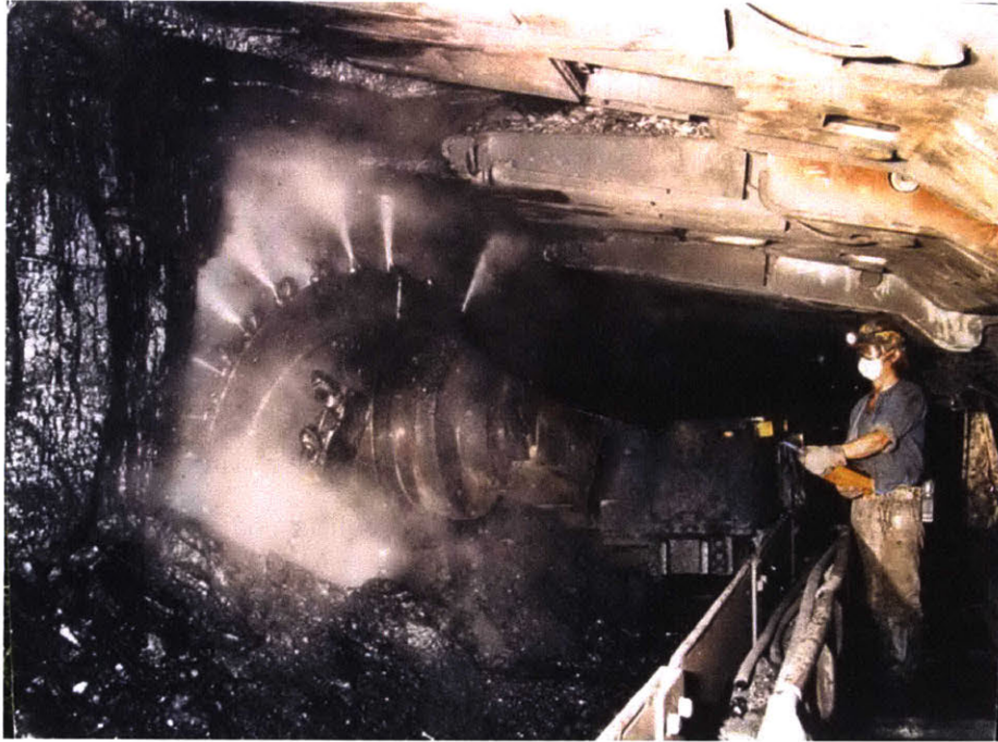
Figure 1-2: A longwall shearer with water sprayers [4]
