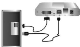
**NOTE:** If using audio, no separate cables are required, as it will be carried over USB.
