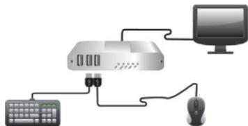
**OPTIONAL:** Connect any additional USB peripherals you wish to use to the Remote unit (install any required software as per the manufacturer's instructions). A powered USB hub may be connected to the Remote unit, if additional USB ports are required.
