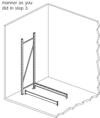
5. Holding the second upright in place, lift the loose ends of the two bottom beams and fit
