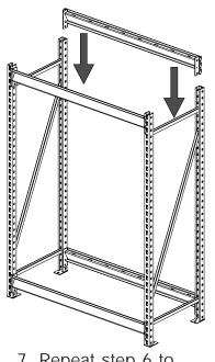
6. Attach the two top beams to the uprights at the desired level, using the same basic principals you used in steps 3 through 5.
