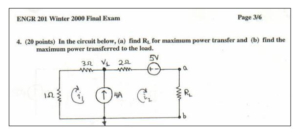
To do this problem, mesh analysis is used to solve for the power transferred as a function of the load,  $R_L$ . Then  $R_L$  is set equal to  $R_{Th}$ , the Thevenin equivalent resistance of the circuit. Four equations are required to solve the problem: two mesh equations, an equation which relates the value of the current source to the mesh currents, and an equation for the power transferred,  $\mathbf{p}$ :
